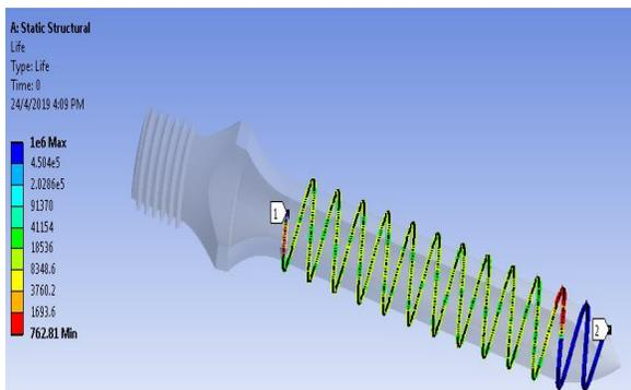
Fig. 10. Life Cycle on path for max load that the CPS can stand (11000 N)
