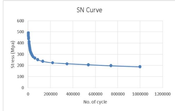
Fig. 11. S-N Curve for CPS life cycle
