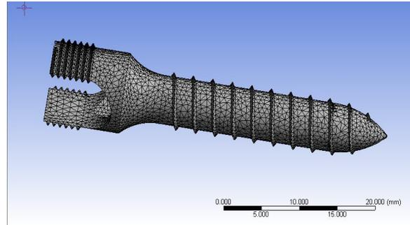
**Fig. 3.** Meshing result using element quality
