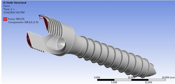
Fig. 5. Force applied on the pedicle screw
