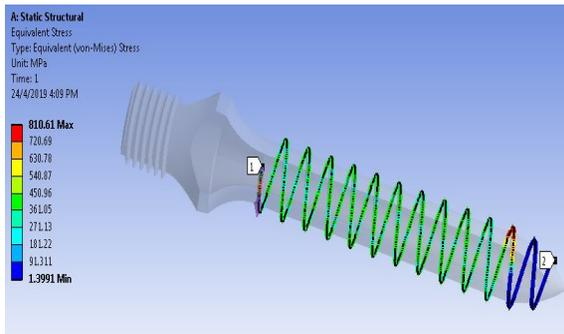
Fig. 9. Von Mises Stress on path for max load that the CPS can stand (11000 N)
