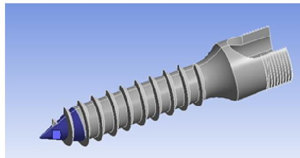
**Fig. 4.** Fixed support being place on the screw tip of the model
