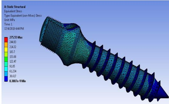
Fig. 8. Von mises stress of commercial design (490.5 N)
