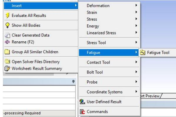
Fig. 6. Inserting of fatigue tool
