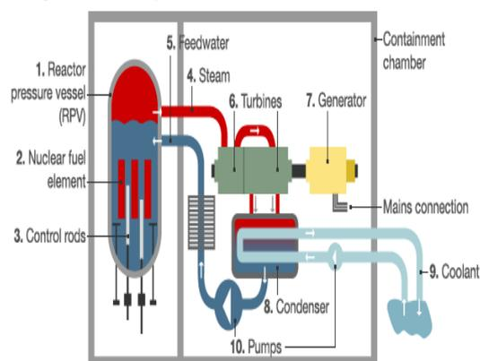
Fig.1 Boiling Water Reactor System
