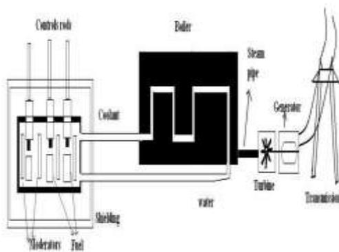
Fig.2 Parts Of Nuclear Plant
