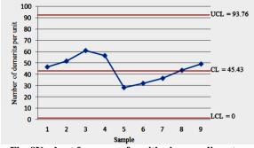
Fig. 8U- chart for nonconformities in pore diameters
