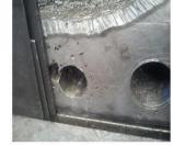
(a) Slag inclusion on the side of plate 7and(b) Porosity on the surface of plate 4
