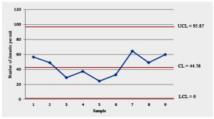
Fig. 7U- chart for nonconformities in pore depths
