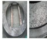
(a) Top surface of the defective drive disc (b) Top surface of the drive disc after first hand grinding
