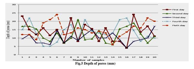
Thus the product in one way can be damaged while exposed to the service as the pores become stress risers and in another way the casts were under size and cannot fit to the required service.
