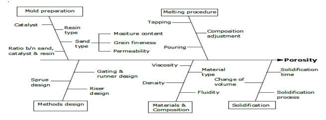
Fig.9Cause and effect diagram of porosity
