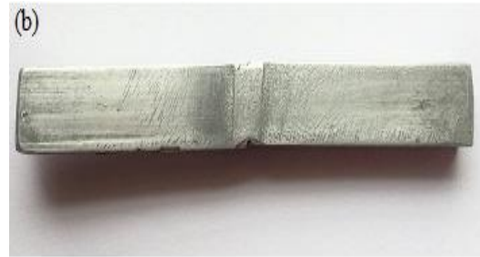
Fig 1: View of microwave processed joint (a) while processing (b) formed joint
