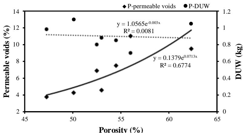
Fig. 10 Relationship between porosity, permeable voids and dry unit mass of composites
