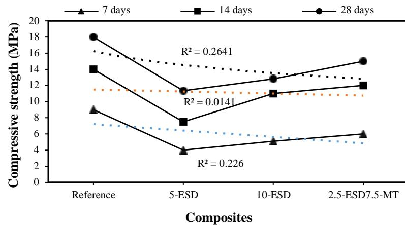
Fig. 12 Compressive strength results of egg shell dust–marble powder–cement paste composites
