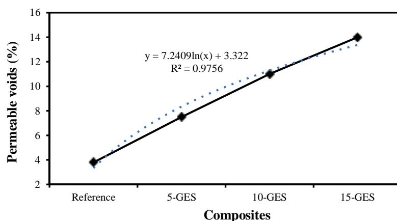
Fig. 6 Permeable voids of granulated egg shell–cement paste composites
