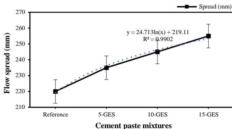
Fig. 5 Flow spread results of granulated egg shell–cement paste mixtures
