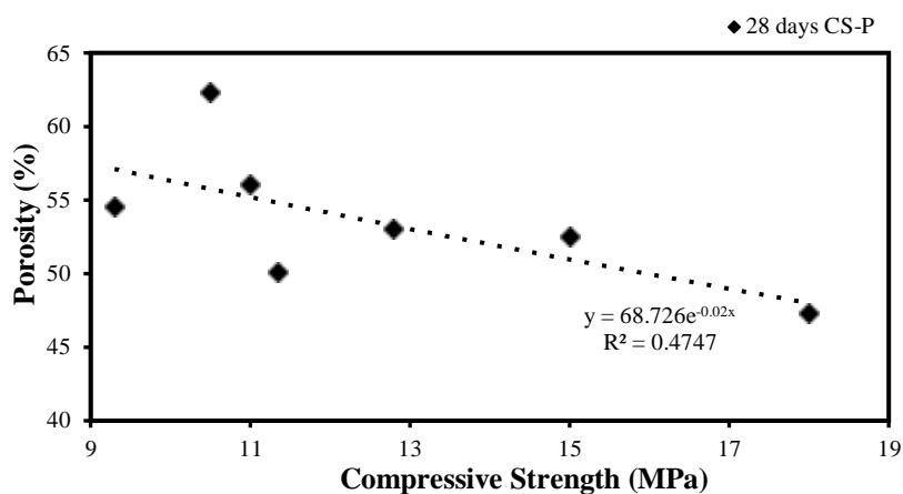
Fig. 13 Relationship between porosity and compressive strength of cement paste composites
