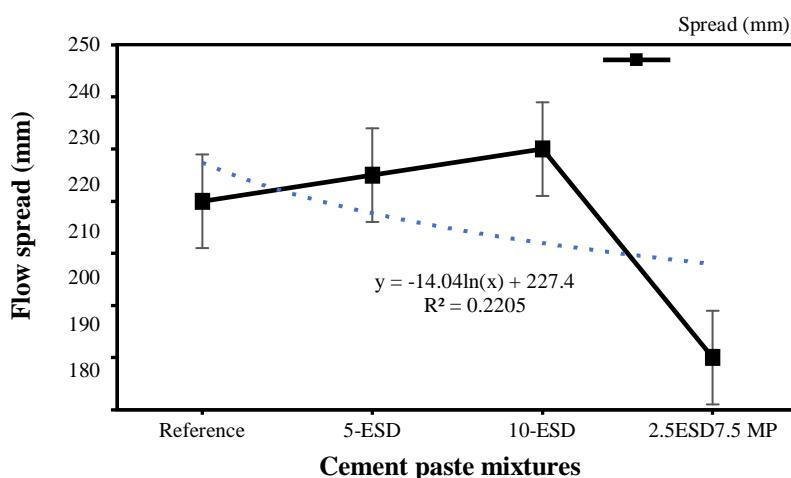
Fig. 4 Flow spread results of egg shell dust–marble powder–cement paste mixtures
