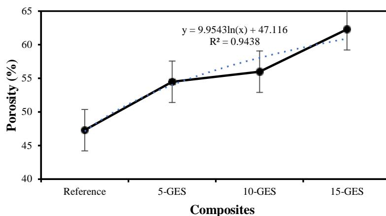
Fig. 8 Porosity results of granulated egg shell–cement paste composites
