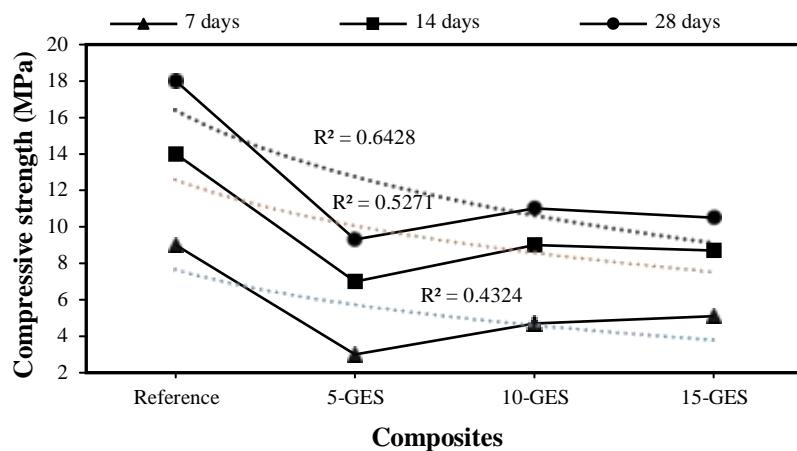
Fig. 11 Compressive strength results of granulated egg shell–cement paste composites
