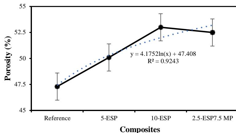
Fig. 9 Porosity results of egg shell dust–marble powder–cement paste composites
