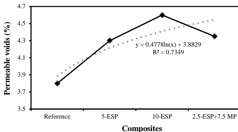
Fig. 7 Permeable voids of egg shell dust–marble powder–cement paste composites
