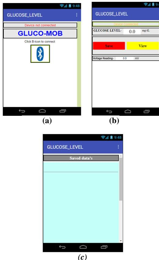
Fig.7. Stages of Second Screen, a- Bluetooth device pairing, b- Glucose value display, c- Saved data display.
