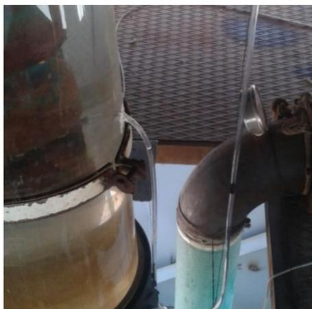
Fig. 2. U-tube differential manometer
