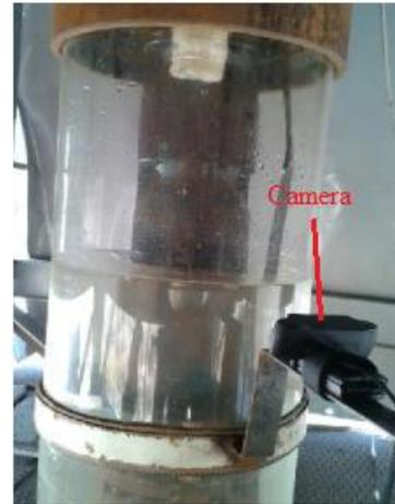
Fig. 3. Submersible pump and connection of the camera
