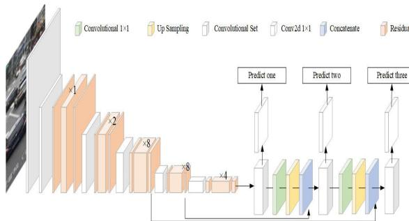
**Figure 3: YOLOv3 Architecture**
