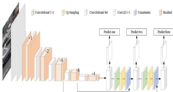
Figure 3: YOLOv3 Architecture
