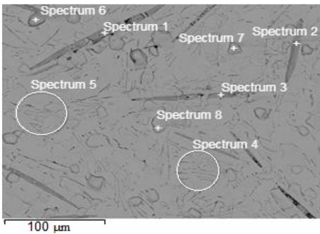
Fig. 7. EDX analysis of Sn1Sr solder
