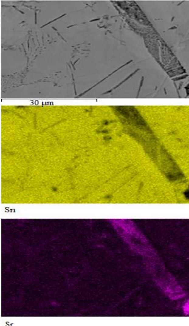
Fig. 6. Distribution of concentration of elements in Sn1Sr solder
