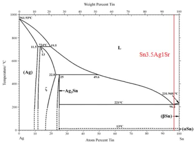
Fig.3 Equilibrium binary diagram of Ag-Sn with a marked concentration of Sn3.5Ag1Sr solder [25]
