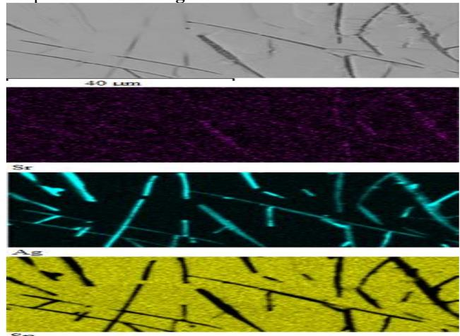
Fig.8. Distribution of concentration of elements in Sn3.5Ag1Sr
