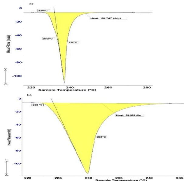
**Fig. 1. a) DTA analysis of specimen No.1 - soldering alloy Sn1Sr; b) DTA analysis of specimen No.2 – soldering alloy Sn3.5Ag1Sr**
