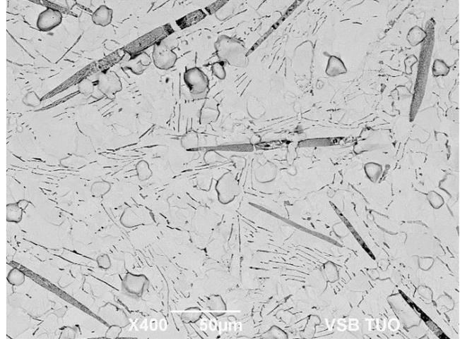
Fig. 4. Microstructural SEM analysis of Sn1Sr solder
