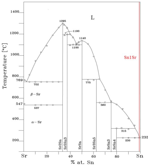
Fig. 2. Equilibrium binary diagram of Sr-Sn with a marked concentration of Sn1Sr solder [24]
