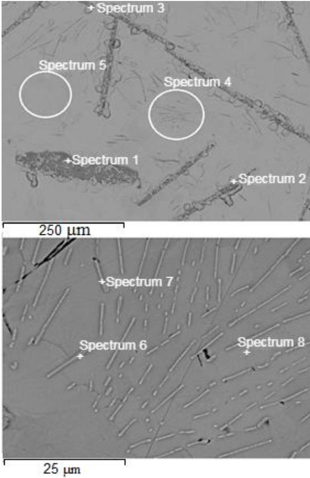
Fig.9. EDX analysis of Sn3.5Ag1Sr solder
