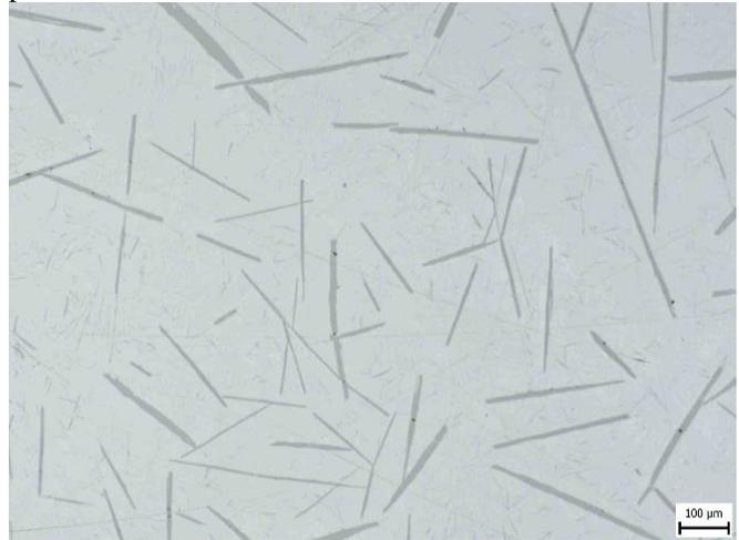
Fig. 5. Microstructural analysis of Sn3.5Ag1Sr solder performed by the light microscopy
