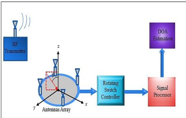
Fig. 2 Block Diagram of DOA Estimation
