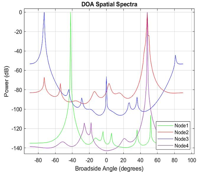
Fig. 9. The spatial spectrum of the second estimation for the four RF nodes
