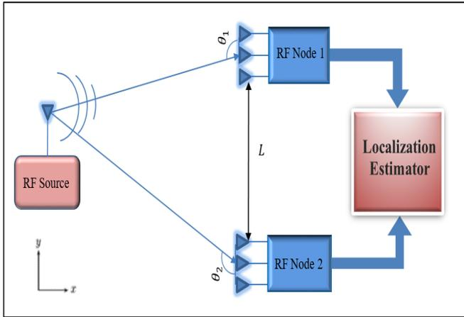
Fig. 3 Block diagram of the triangulation process
