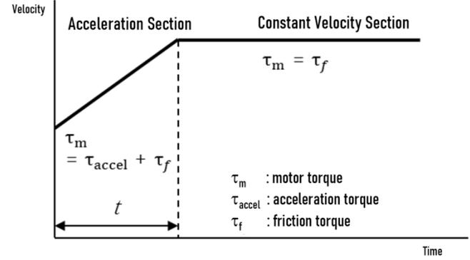
**Fig. 6 Required Motor Torque**
