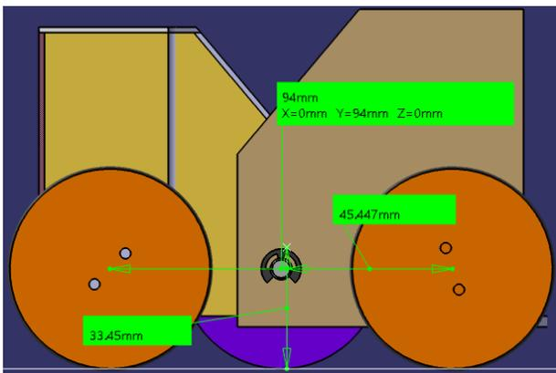
**Fig. 5. Design Parameter from Center of Gravity**
