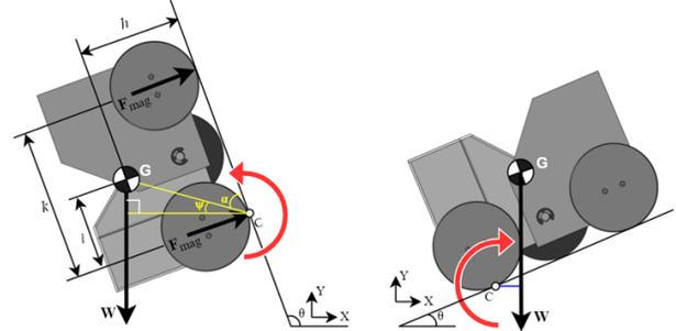
**Fig. 11 Moment Chang due to Climbing Angle at Joint axis**
