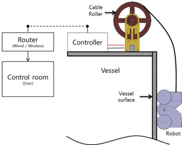
**Fig.1 System Configuration**
