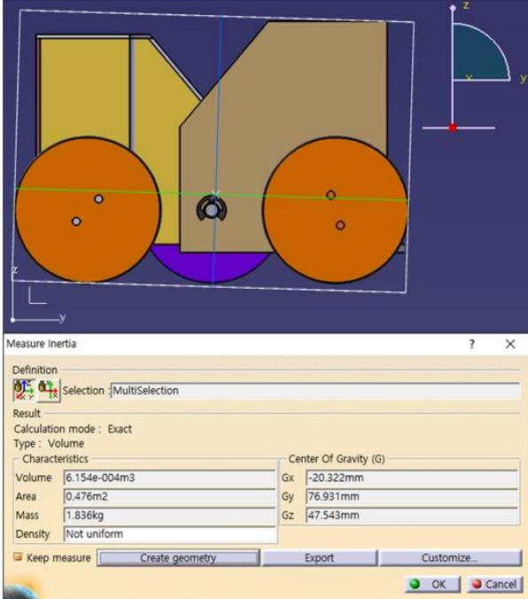
**Fig 4. Center of Gravity in Wall Climbing Robot**
