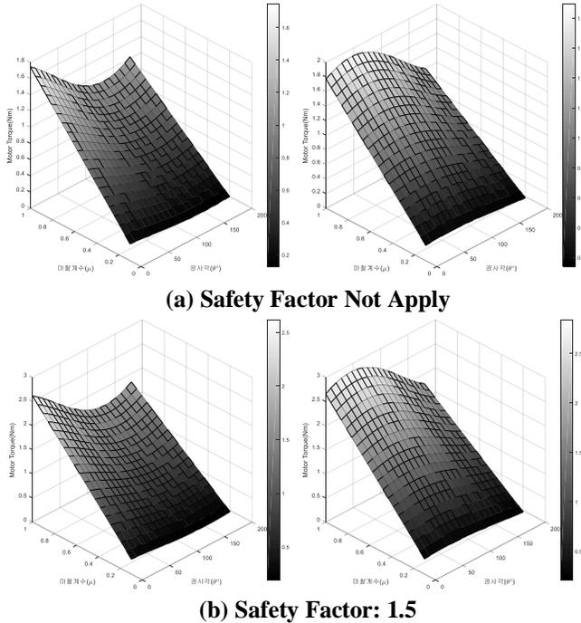
**Fig. 7 Result of Driving Torque (Left: Front, Right: Rare)**
