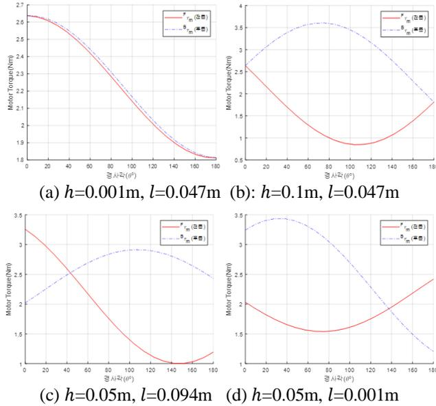
**Fig. 10 Result of Driving Torque by Changing Center of Gravity**
