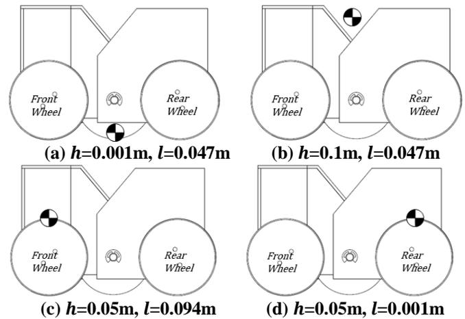
**Fig. 9 Changing Center of Gravity in Design Parameter**
