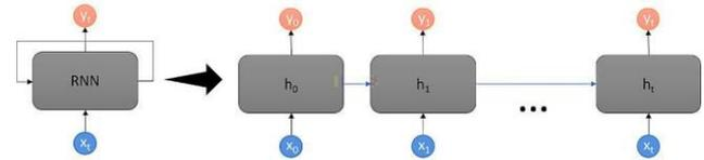
Fig. 10 An RNN cell is unrolled one at a time.
