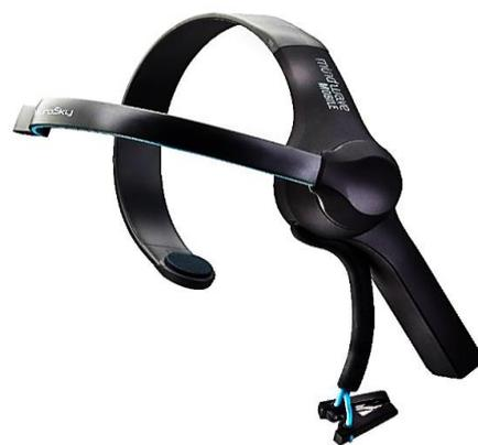
Fig. 2 Neurosky MindWave Single-Channel EEG Headset
