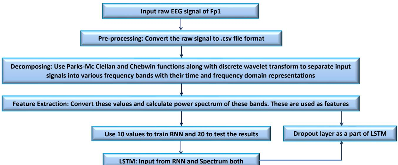
Fig. 16 The flowchart of the proposed RNN-LSTM combined for mental stress detection
