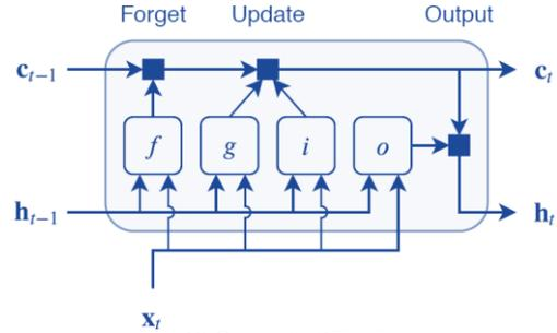
Fig. 13 Gates of LSTM Layer
