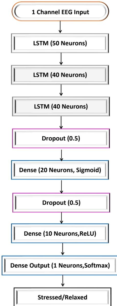
Fig. 15 Flowchart for LSTM with dropout layer
