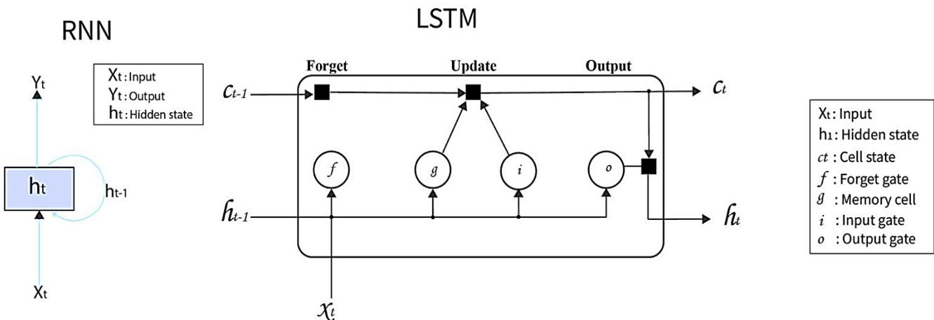
Fig. 14 b) RNN-LSTM Network layer
