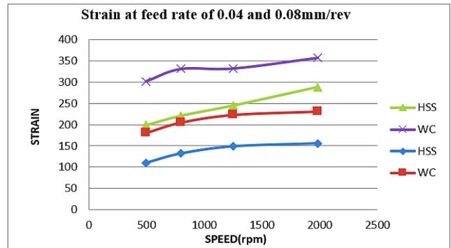
Fig. 11 Speed and feed relationship with Strain
