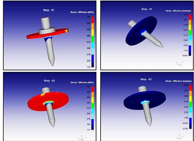
Fig. 5 Stress, strain analysis of HSS tool on AL6061-T6 workpiece at Feed 0.08mm/rev and Speeds 1980 & 1250rpm
