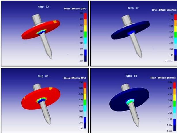
Fig. 8 Stress, strain analysis of Tungsten Carbide tool on AL6061-T6 workpiece at Feed 0.04 mm/rev and Speeds 1980 & 1250rpm
