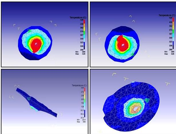
Fig. 9 Temperature distribution and deformation at various speeds and feed rates with HSS and Tungsten carbide tools.
