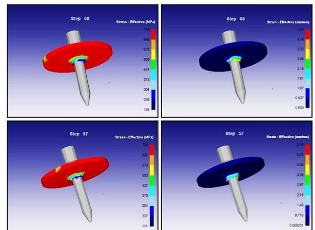
Fig. 7 Stress, strain analysis of Tungsten Carbide tool on AL6061-T6 workpiece at Feed 0.08mm/rev and Speeds 1980 & 1250rpm
