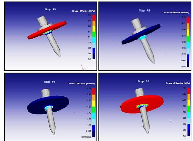
Fig. 6 Stress, strain analysis of HSS tool on AL6061-T6 workpiece at Feed 0.04mm/rev and Speeds 1980 & 1250rpm.
