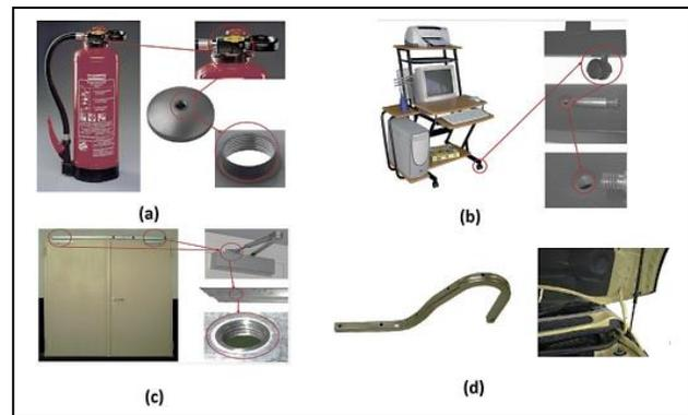
Fig. 2 Applications of Friction Drilling Process
