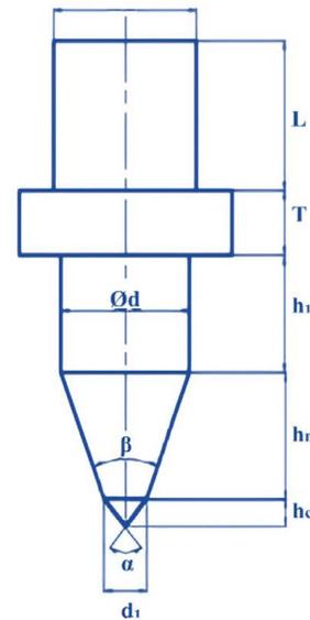
Fig. 3 Friction Drilling Tool
