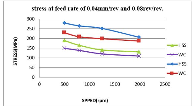
Fig. 10 Speed and feed relationship with stress
