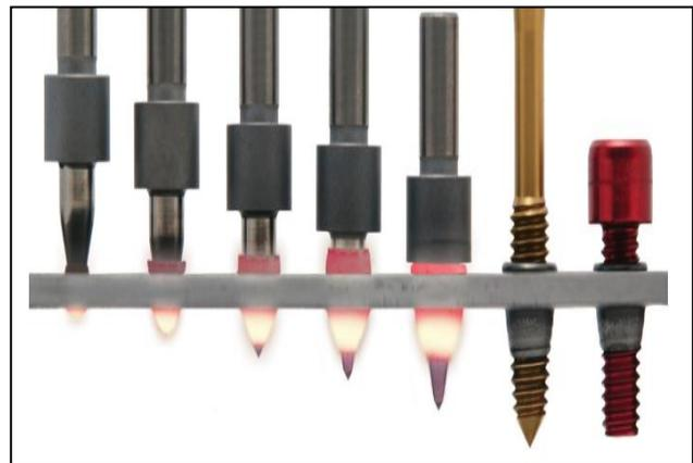
Fig. 1 Various stages of the Friction Drilling Process.
