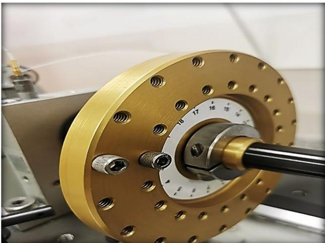
Fig. 4 The imbalance condition is simulated by installing two pieces of 1/4-20 socket head cap screws
