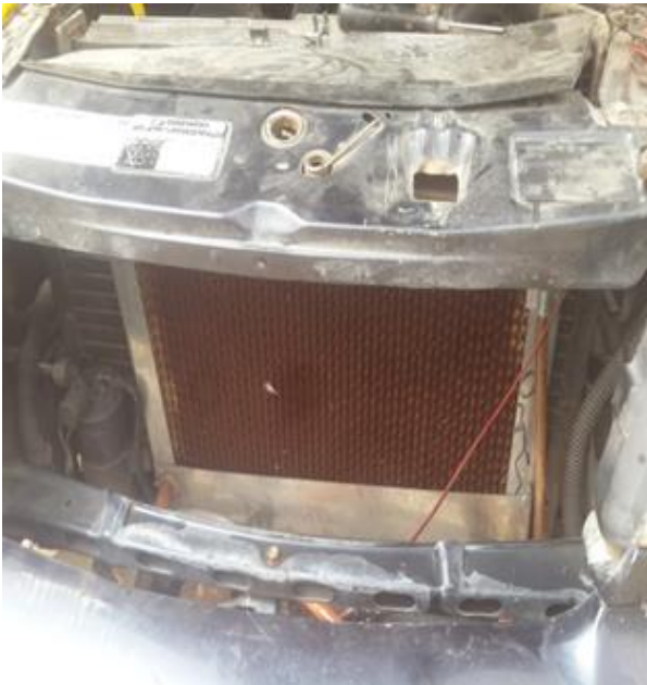
Fig. (5-b) Cellulose pad installed in the car
