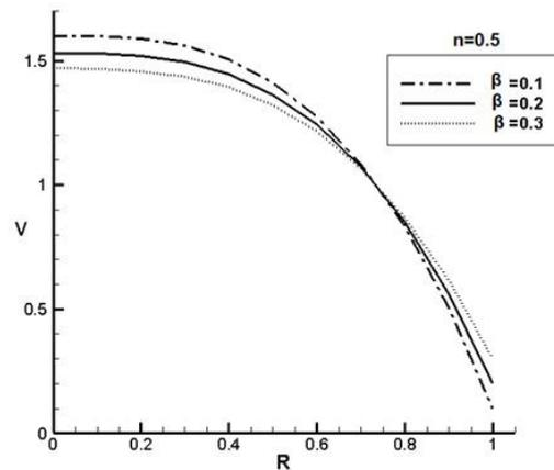
Fig. 5 Velocity profiles of slip flow through microchannel for different slip co-efficient
