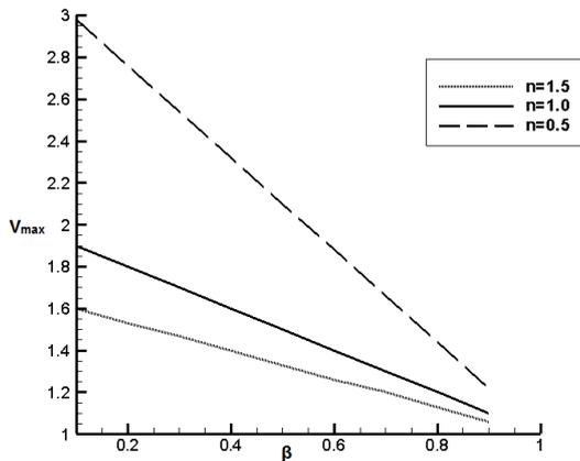
Fig. 7 Comparison of developed maximum velocity ( $V_{max}$ ) and Slip Coefficients ( $\beta$ )
