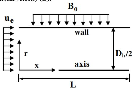
Fig. 1 Fluid domain of circular microchannel with the externally applied magnetic field ( $B_0$ )
