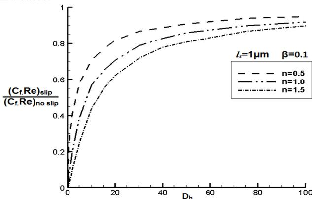
Fig. 8 Effect of hydraulic diameter ( $D_h$ ) on Poiseuille No. ( $C_f Re$ )
