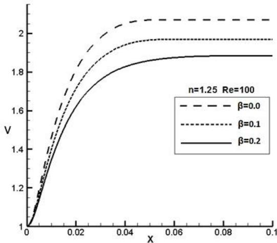
Fig. 3 Comparison of centerline velocities for different Slip Co-efficient ( $\beta$ )
