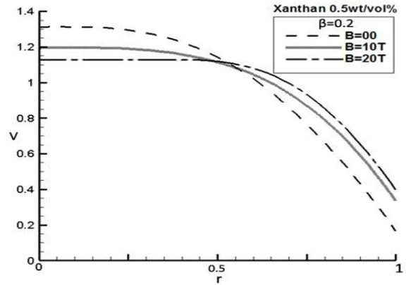
Fig. 9 the effect of the externally applied magnetic field on velocity profiles
