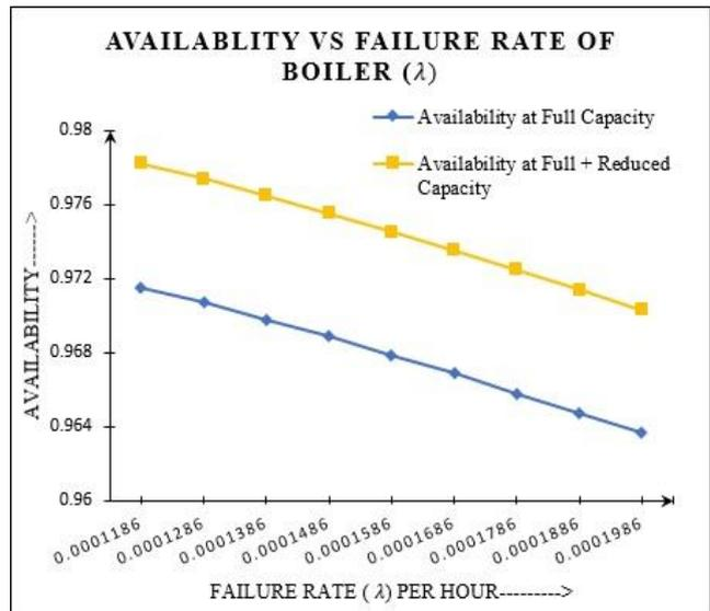
**Fig. 3 Availability vs. Failure rate of the boiler**
