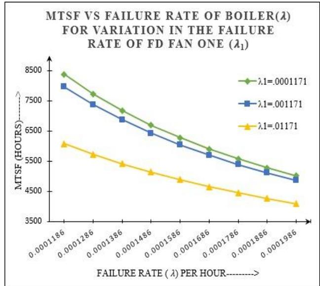
**Fig. 2 MTSF vs. Failure rate of the boiler**
