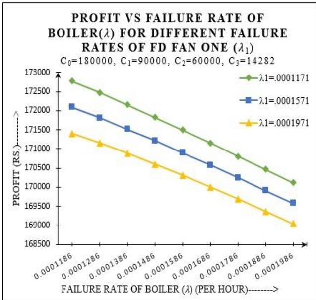
**Fig. 4 Profit vs. Failure rate of the boiler**
