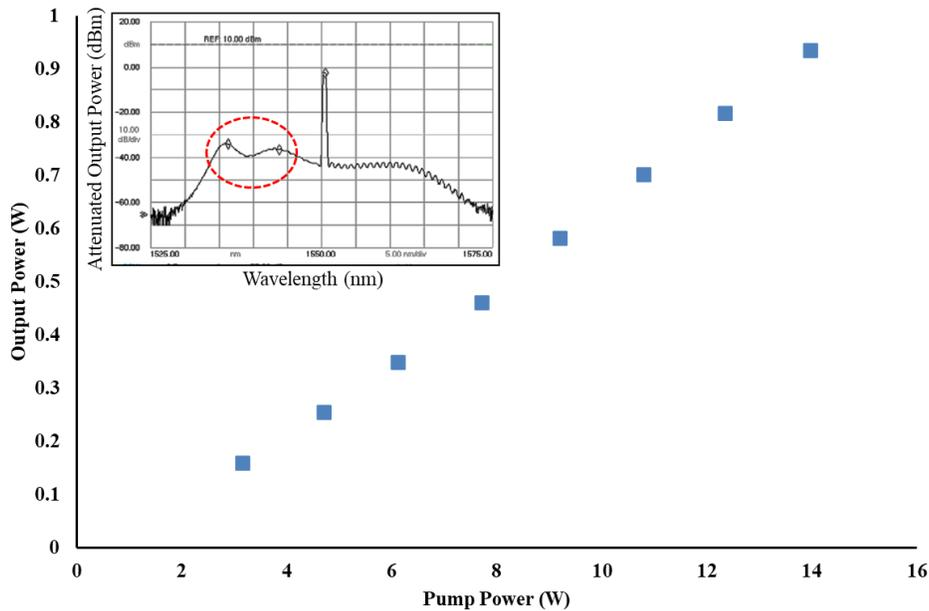
Fig. 8 Output power of the amplified signal for different pump power values obtained from Fiber 4
