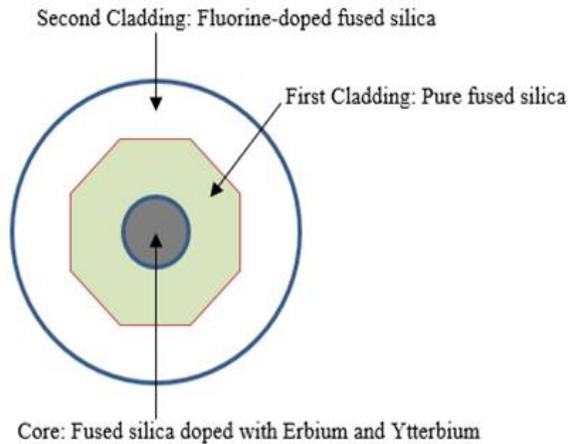
Fig. 1 Illustration of a dual clad fiber with octagonal inner cladding
