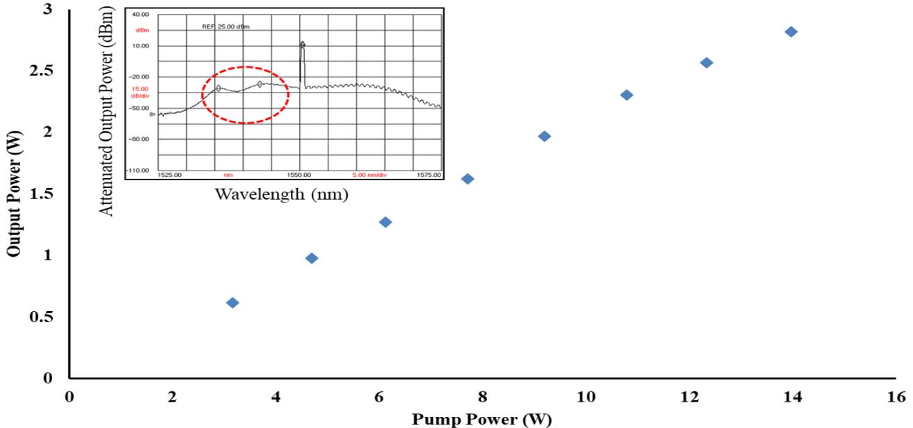
**Fig. 5 Output power of the amplified signal for different pump power values obtained from Fiber 1**
