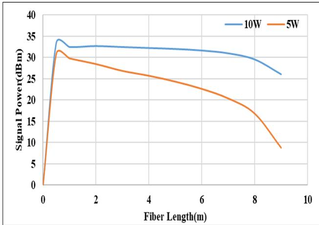
Fig. 3 Simulation result for the fiber length optimization with Opti System tool
