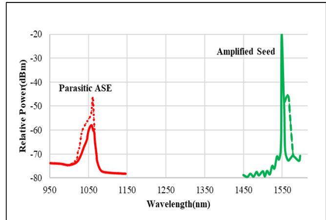
Fig. 2 Emission Spectrum of Er-Yb Co-doped Fiber
