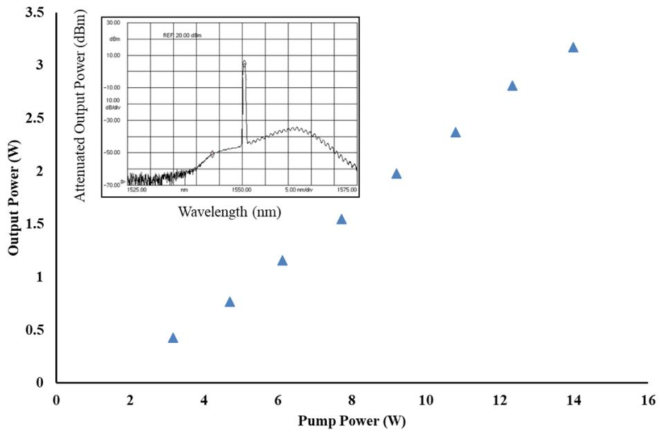
Fig. 7 Output power of the amplified signal for different pump power values obtained from Fiber 3
