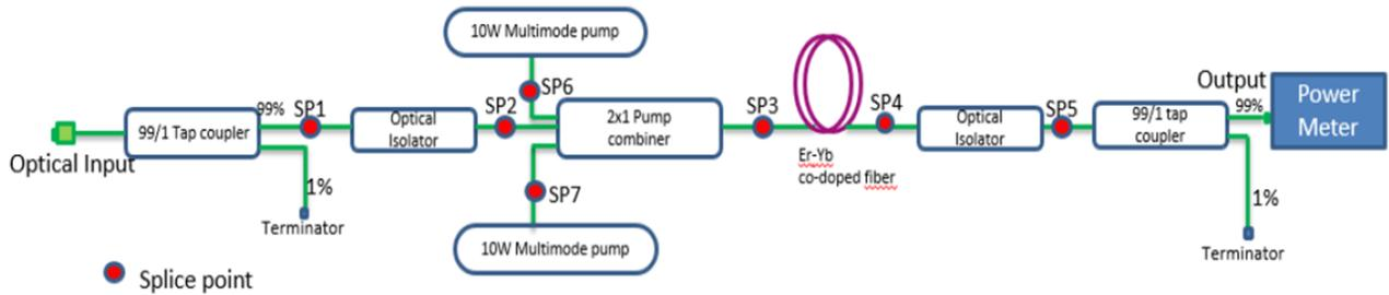
Fig. 4 Architecture of a high power amplifier with Er-Yb Co-doped Fiber
