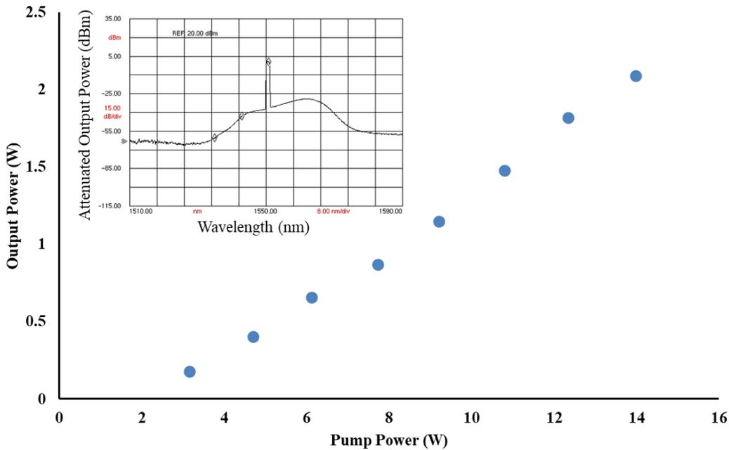
Fig. 6 Output power of the amplified signal for different pump power values obtained from Fiber 2
