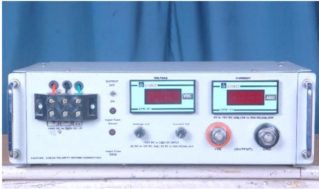
Fig. 3 Power Conditioning System
