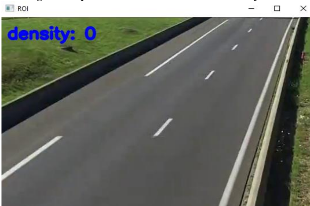
Fig. 11 Sample Result Frame with 0 traffic density value
