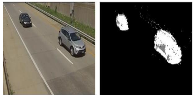
Fig. 6 Sample frame and Vehicle Detection after Masking
