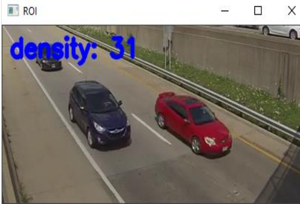
Fig. 9 Sample Result Frame with 31 traffic density value
