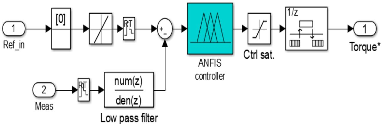
Fig. 11 ANFIS torque regulator
