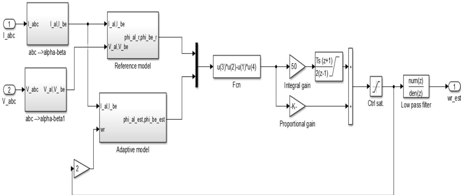
Fig. 10 MRAS speed estimator internal modeling
