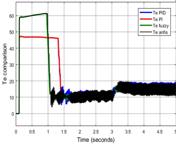
Fig. 16 IM torque comparison of all controllers (PID, PI, fuzzy, and ANFIS)
