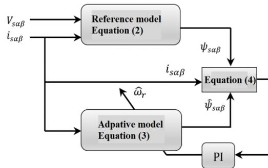
Fig. 2 MRAS machine speed estimator
