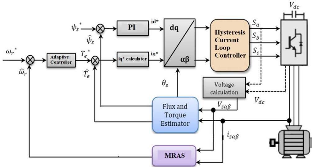
Fig. 1 IFOC control of IM with MRAS module for speed estimation
