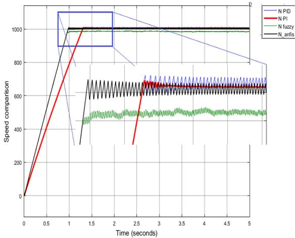
Fig. 17 IM Speed comparison of all controllers (PID, PI, fuzzy, and ANFIS)
