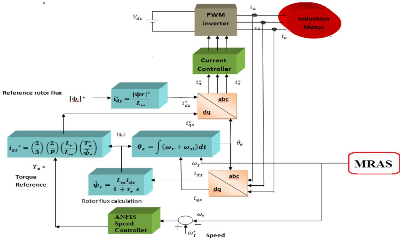
Fig. 3 IFOC control scheme with ANFIS speed controller
