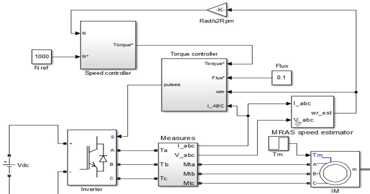
Fig. 9 Simulation modeling of proposed IM drive
