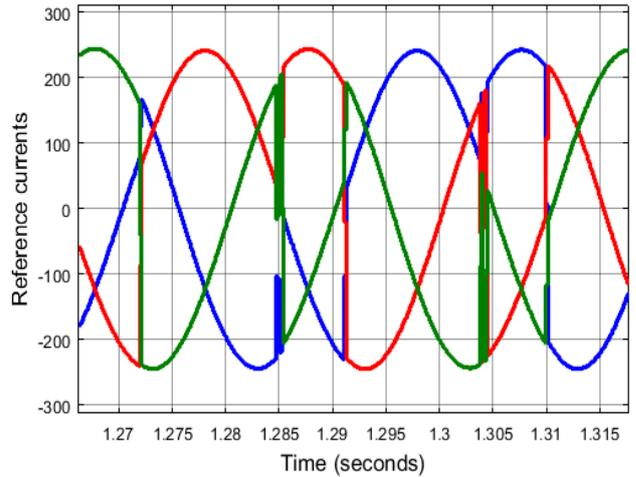
Fig. 14 Reference currents from the IFOC scheme
