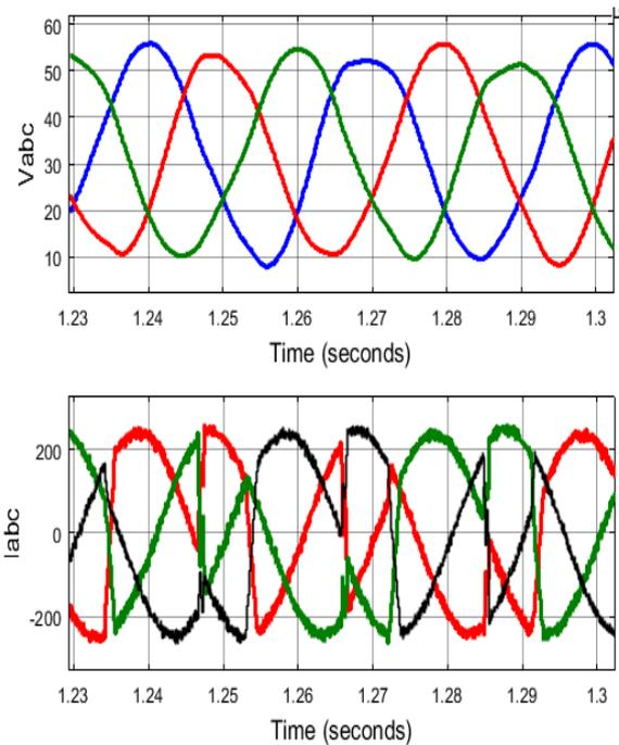
Fig. 15 Stator voltages and currents
