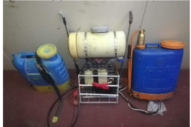
Fig. 8 Fumigation backpacks with the fumigation module
