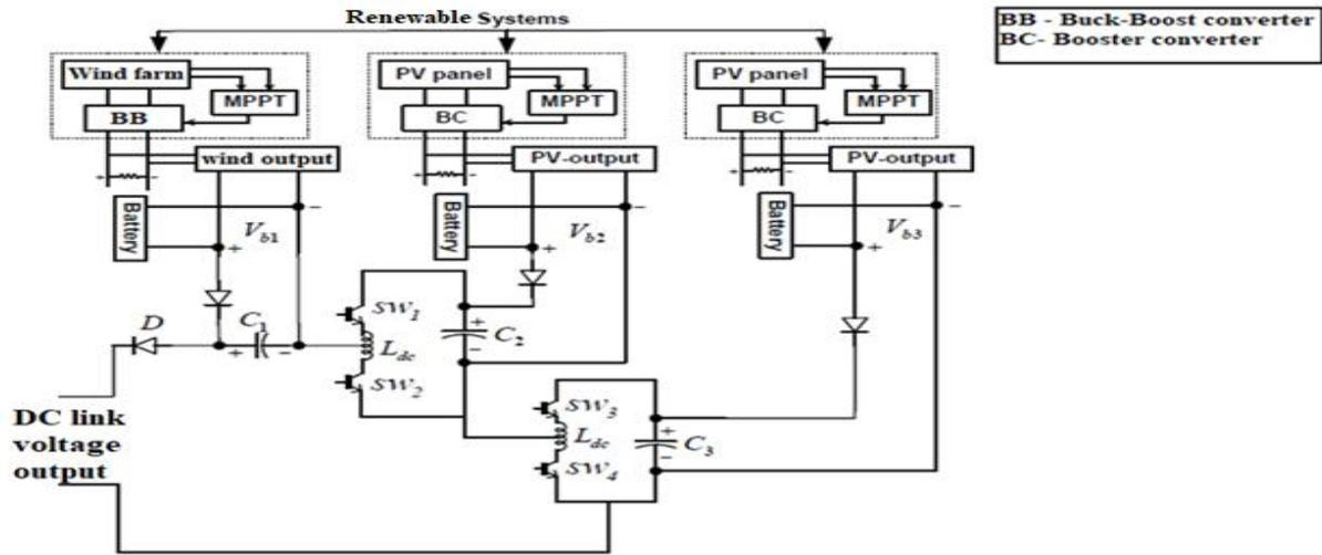
Fig. 2 RSC-MLC module with hybrid renewable sources
