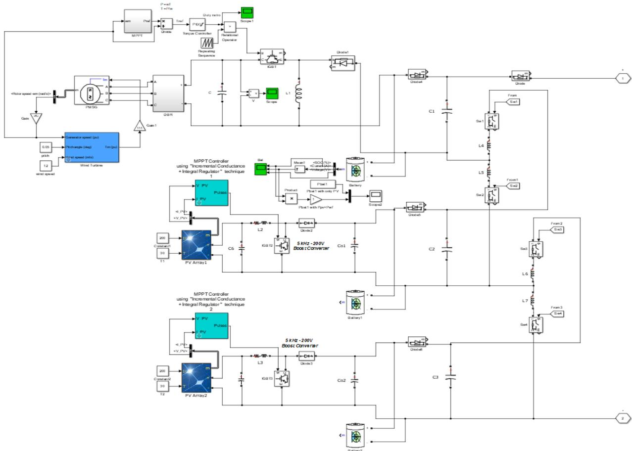
Fig. 6 Hybrid renewable source RSC-MLC module
