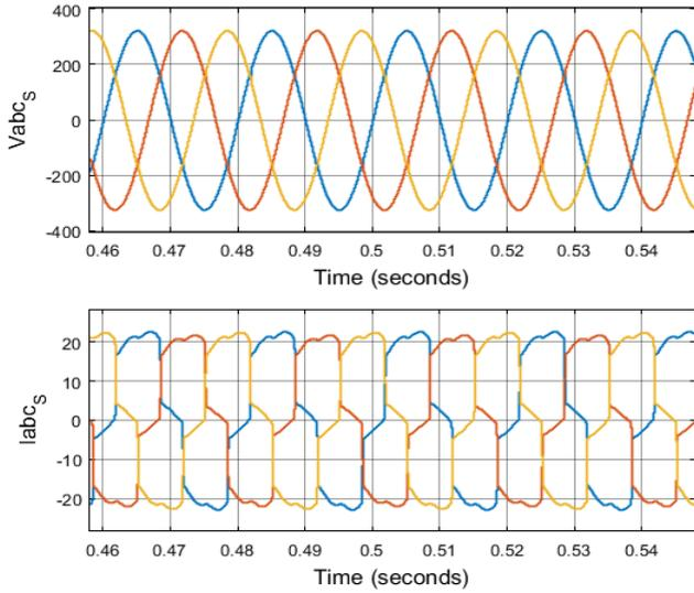
**Fig. 8** Voltages and currents of the three-phase source without D-STATCOM
