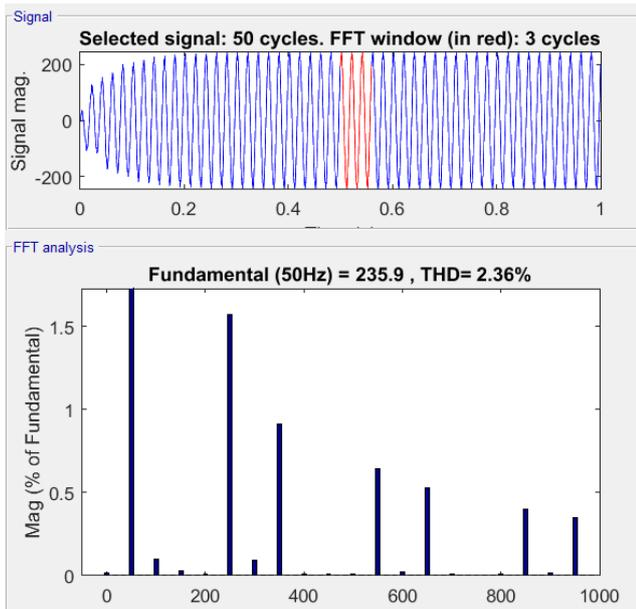
Fig. 13 FFT analysis of source current to determine THD
