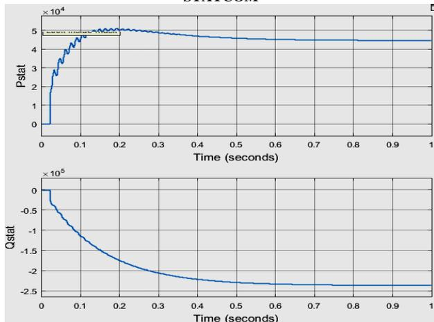
**Fig. 10** Injected active and reactive power of D-STATCOM
