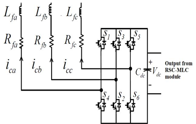
Fig. 4 D-STATCOM schematic
