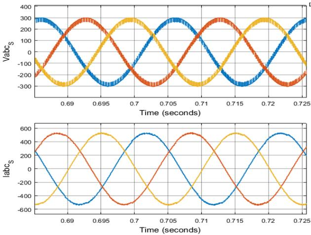
**Fig. 9** Voltages and currents of the three-phase source without D-STATCOM
