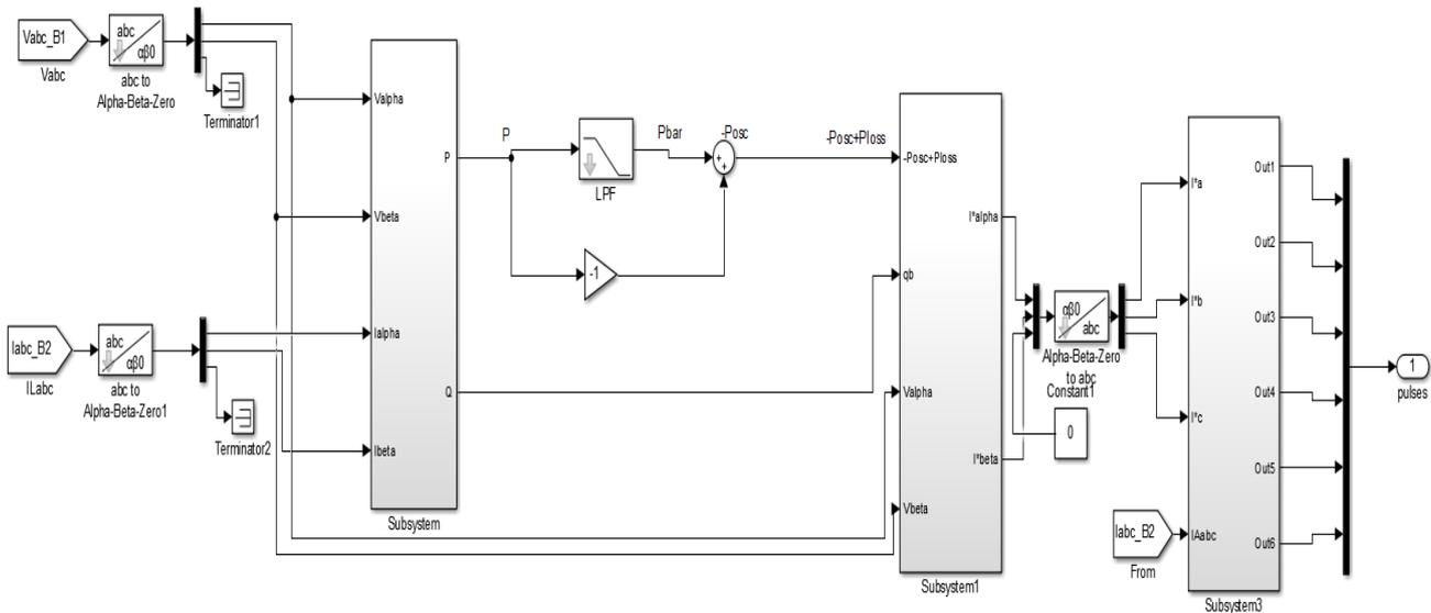
Fig. 7 PQ theory D-STATCOM controller
