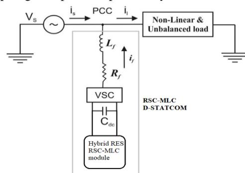
Fig. 1 Proposed test system with hybrid renewable source RSC-MLC module
