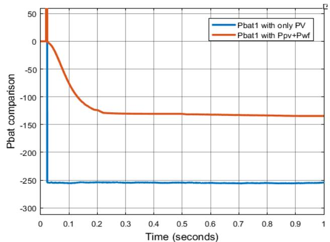
**Fig. 12** Comparative battery storage power with only PVA module and hybrid wind farm and PVA module
