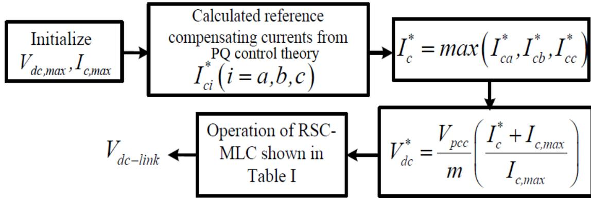
Fig. 3 Reference DC link voltage controller
