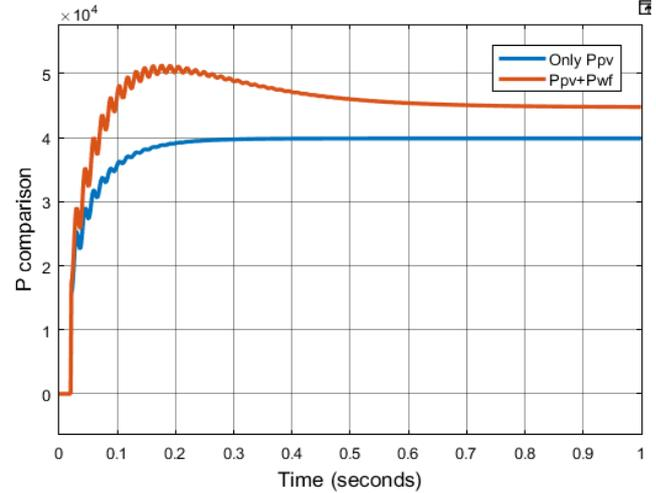
**Fig. 11** Comparative active power with only PVA module and hybrid wind farm and PVA module
