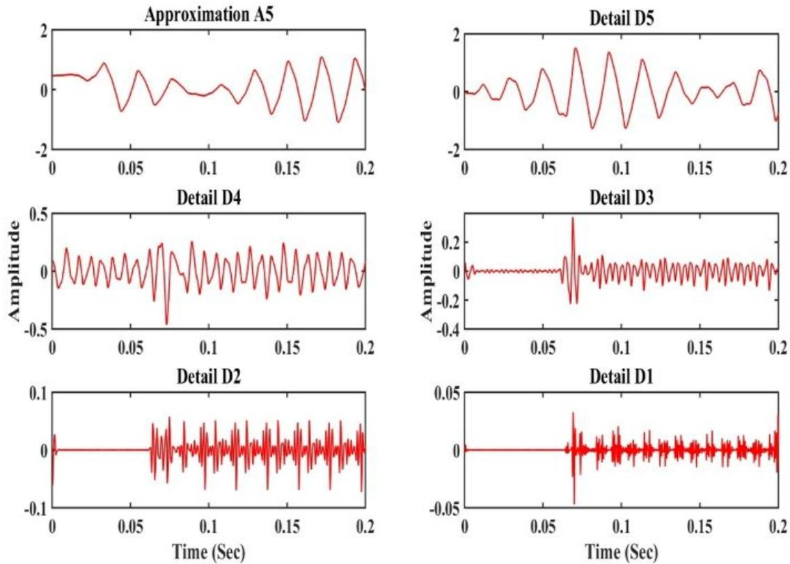
**Fig. 8 DWT Output of Non-linear load switching**
