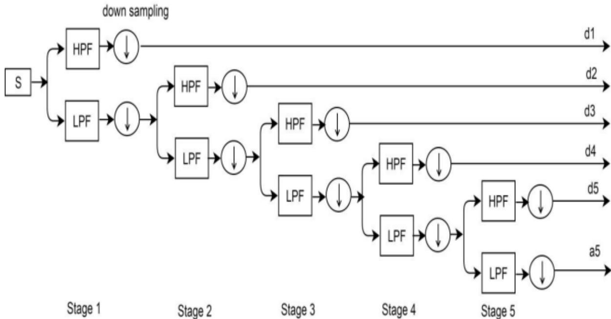
Fig. 6 Discrete Wavelet Transform - Five Level
