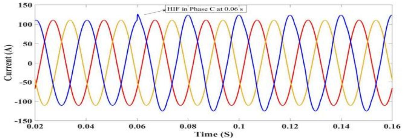
Fig. 5 High Impedance Fault current signal
