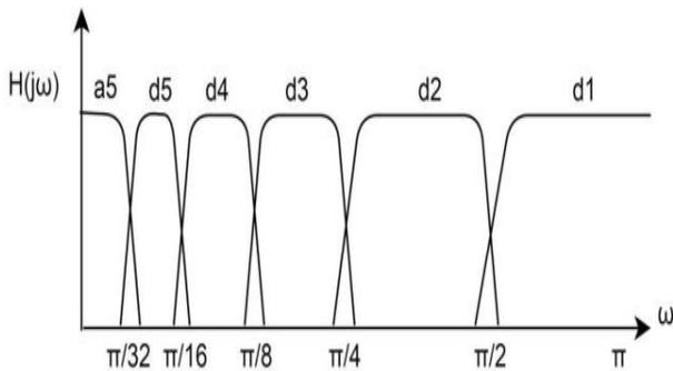
Fig. 7 Five Level Frequency Band of DWT
