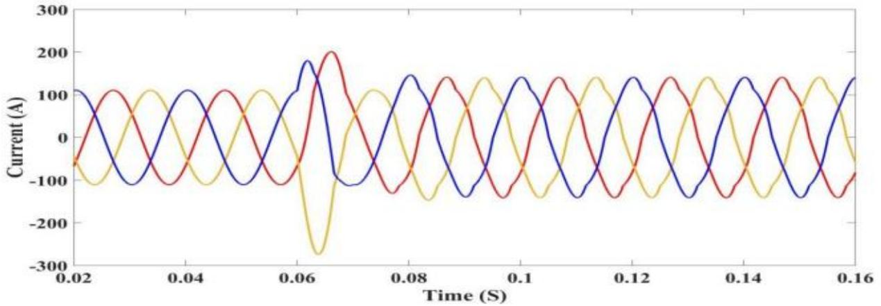
Fig. 3 Non-Linear load switching current signal
