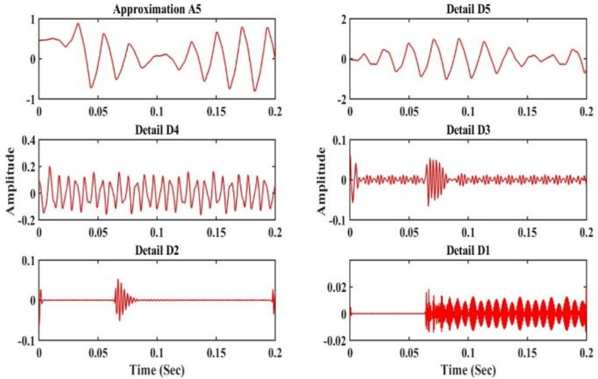
Fig. 9 DWT Output of Capacitance Switching
