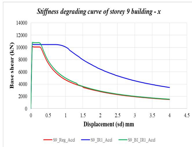
Fig. 10 Stiffness degradation curve for different storey 9 building case
