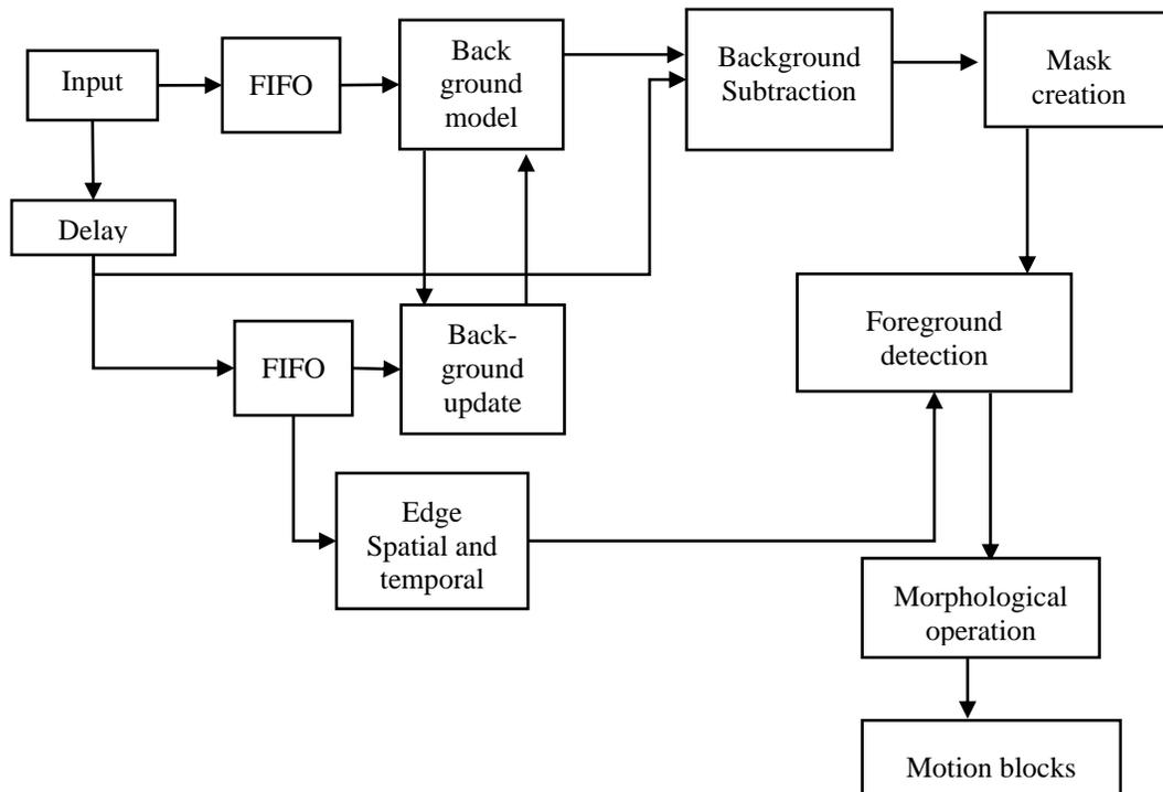
Fig. 2 Block diagram for FPGA implementation of proposed moving object detection
