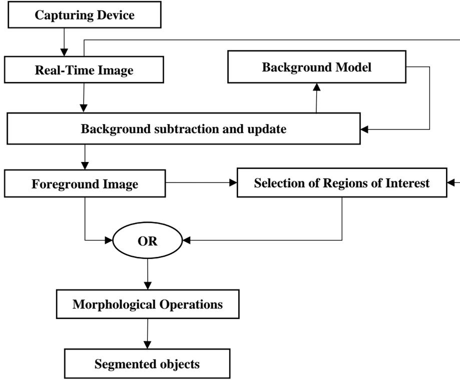
Fig. 1 Block diagram of the motion segmentation process
