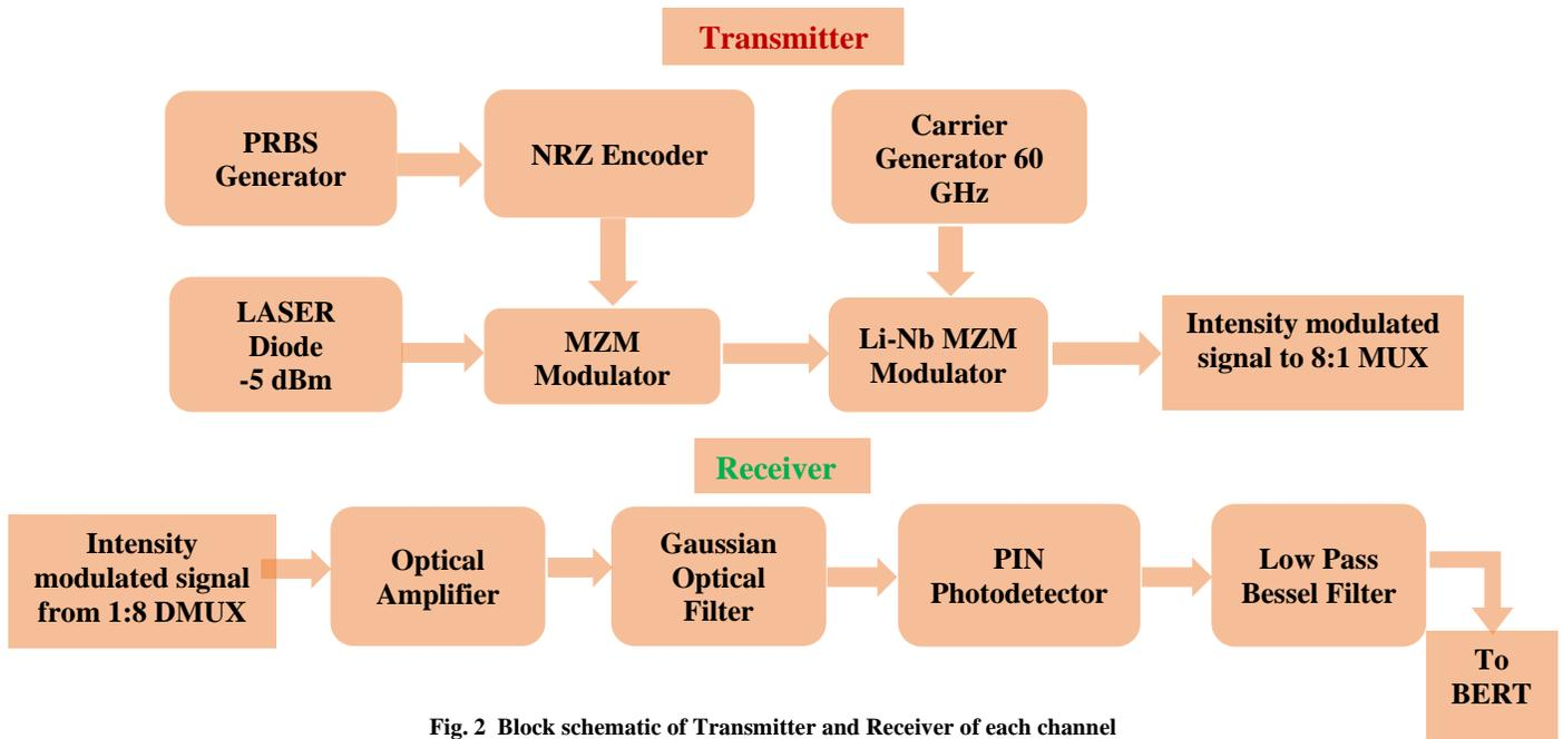
Fig. 2 Block schematic of Transmitter and Receiver of each channel
