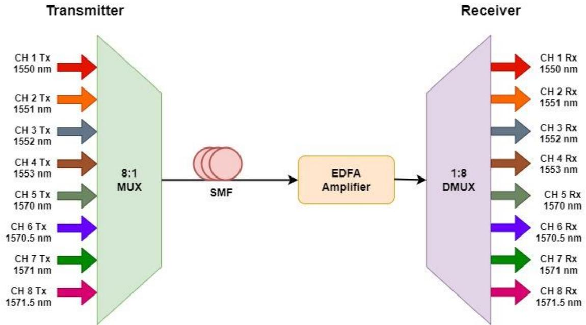
Fig. 1 Generalized block schematic of the proposed method
