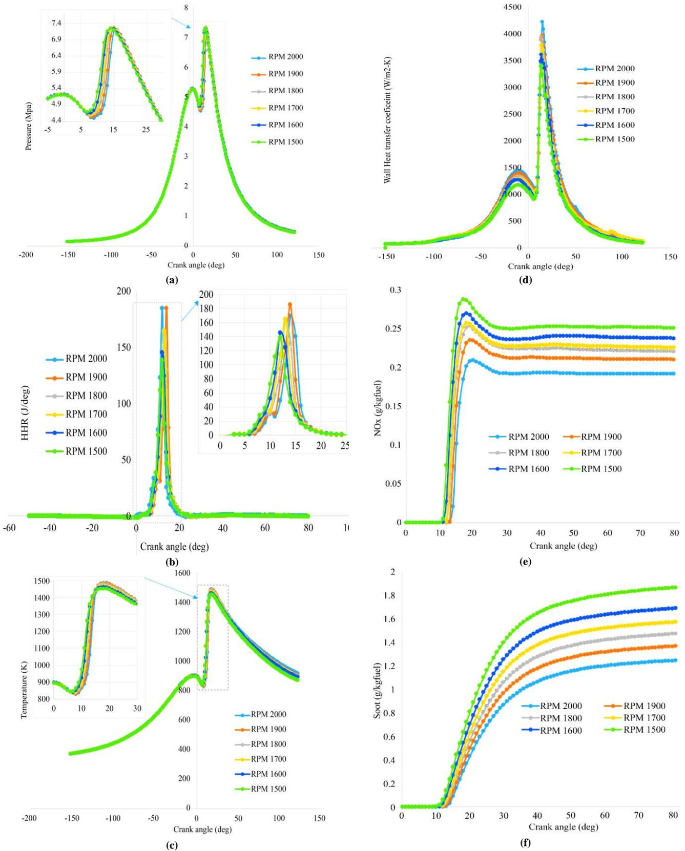
Fig. 4 Variation: Pressure (a), Heat release rate (b), Temperature (c), Wall heat transfer (d), Nox (e), soot (f).
