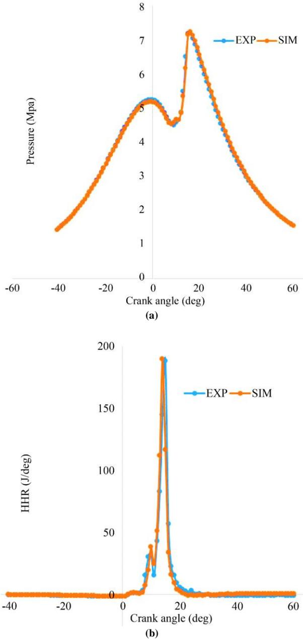
Fig. 3 Model validation: (a) Validation of the model for pressure (b) Validation of the model for heat release rate
