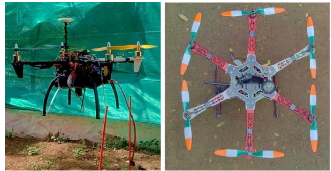
Fig. 3 Sample assembled drone with mounted sprayer and camera
