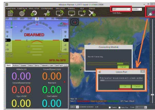
Fig. 4 Connecting mission planner software with Raspberry Pi
