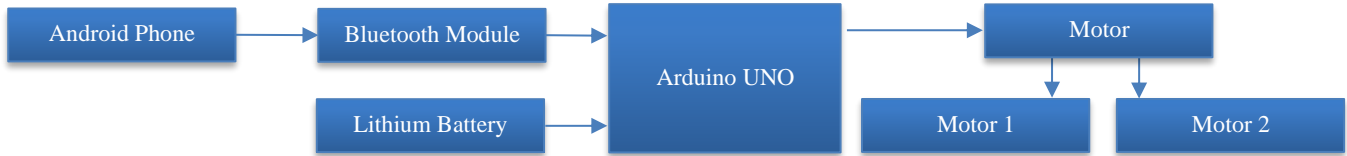
Fig. 9 Boat movement system block diagram
