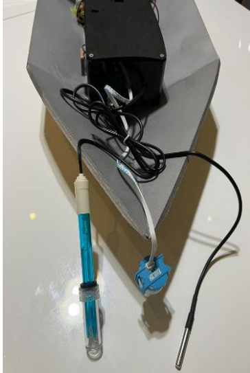
Fig. 13 Instalment of the sensors in the front of the boat
