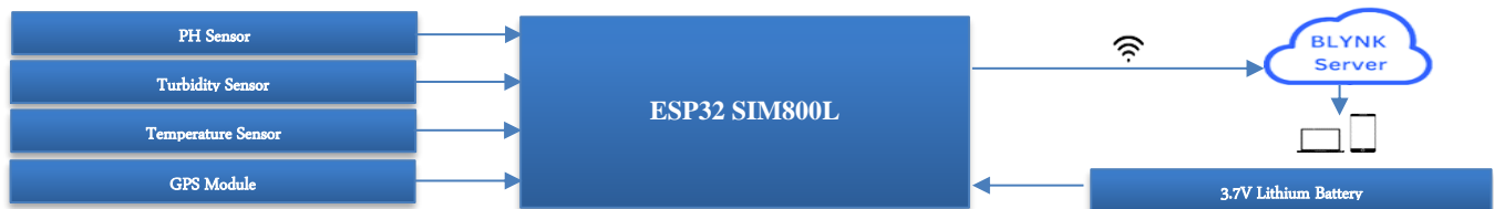
Fig. 6 SWQM system block diagram
