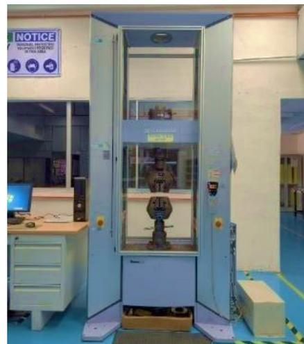
Fig. 3 Using shimadzu Universal Testing Machine (UTM)
