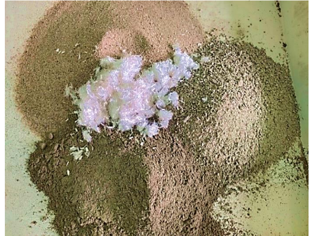
Fig. 5 Glass fiber with CDW
