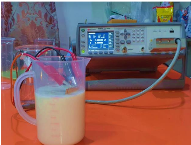
Fig. 2 Measuring the electrical capacity of raw milk using a 2s-ICs
