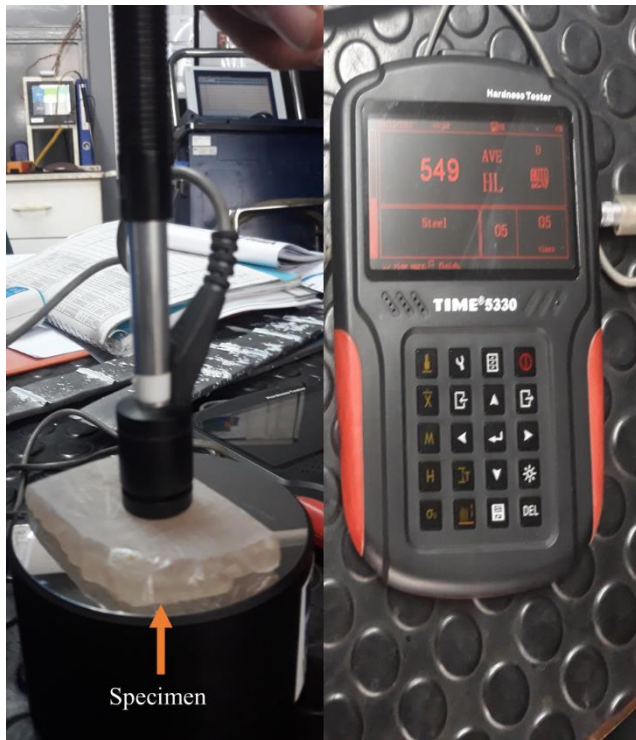
Fig. 4 LEEB hardness testing
