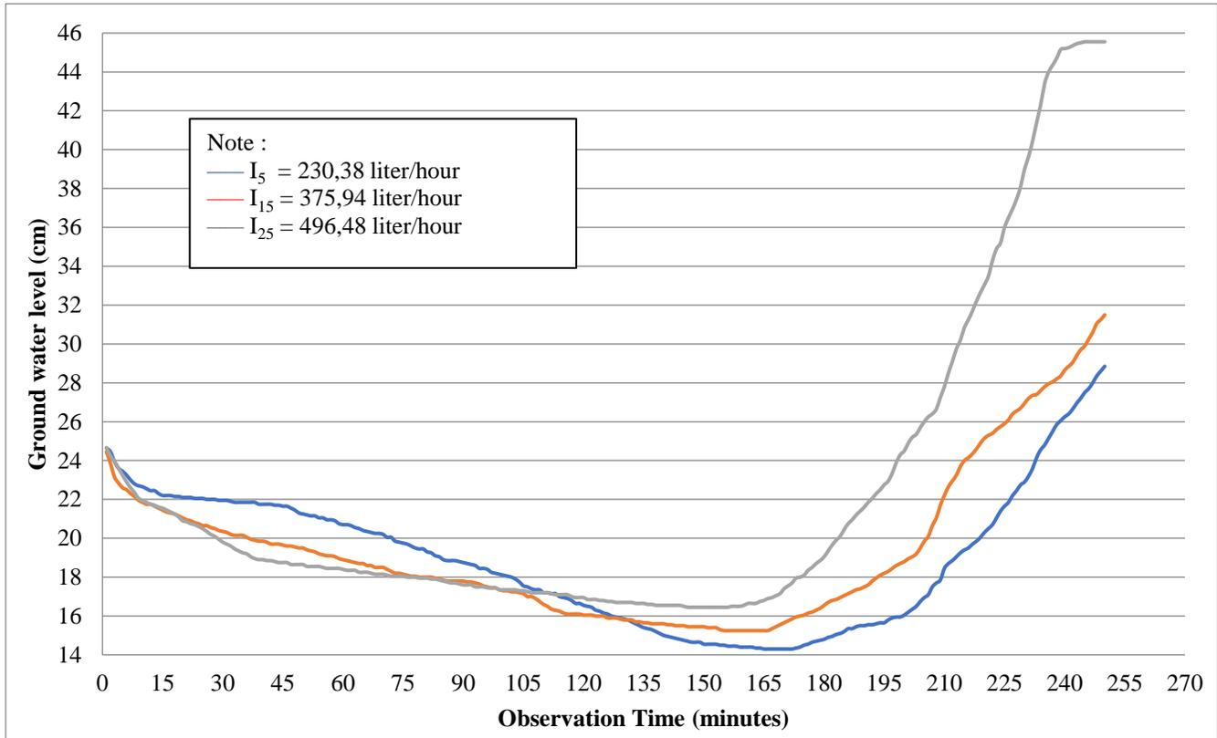
Fig. 2 Groundwater Level Fluctuation on Sandy Silty Clay with Rainfall Intensity Variations I<sub>5</sub>, I<sub>15</sub>, and I<sub>25</sub>
