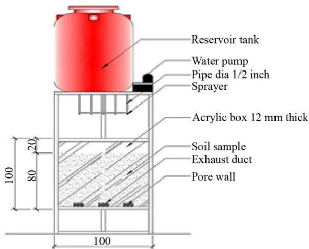
Fig. 1 Capillary Shock Test Model Tool
