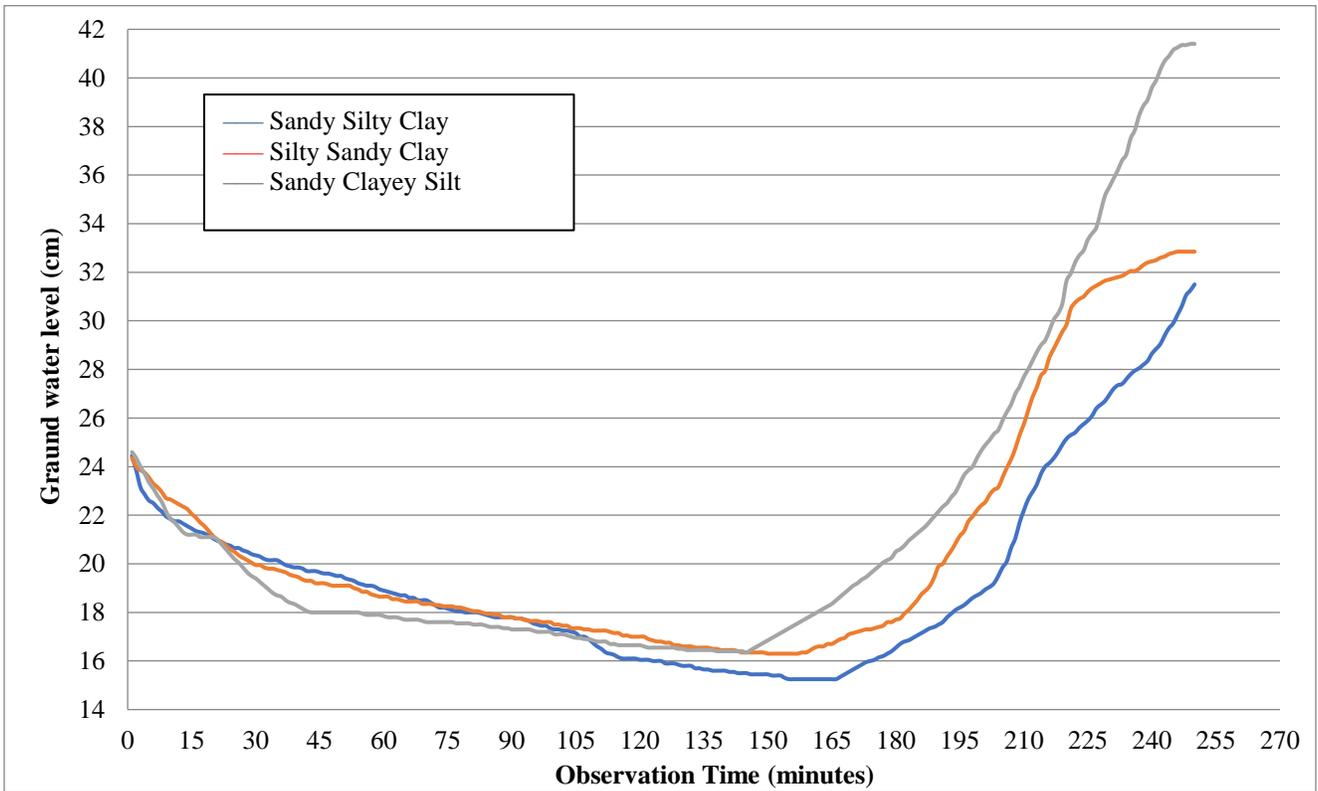
Fig. 6 Groundwater Level Fluctuations in 3 Types of Fine-Grained Soil with Rainfall Intensity  $I_5$
