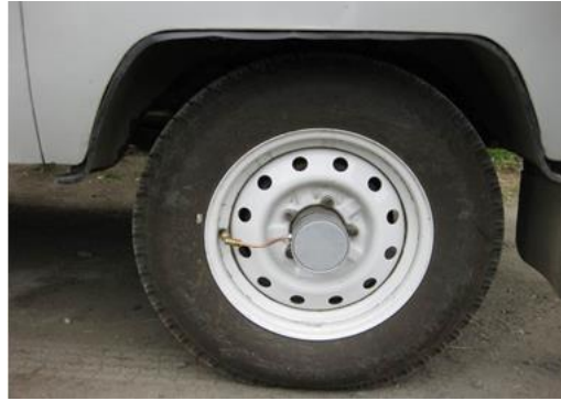
Fig. 7 Automatic device for maintaining normal tire pressure installed on the UAZ-2206 car
