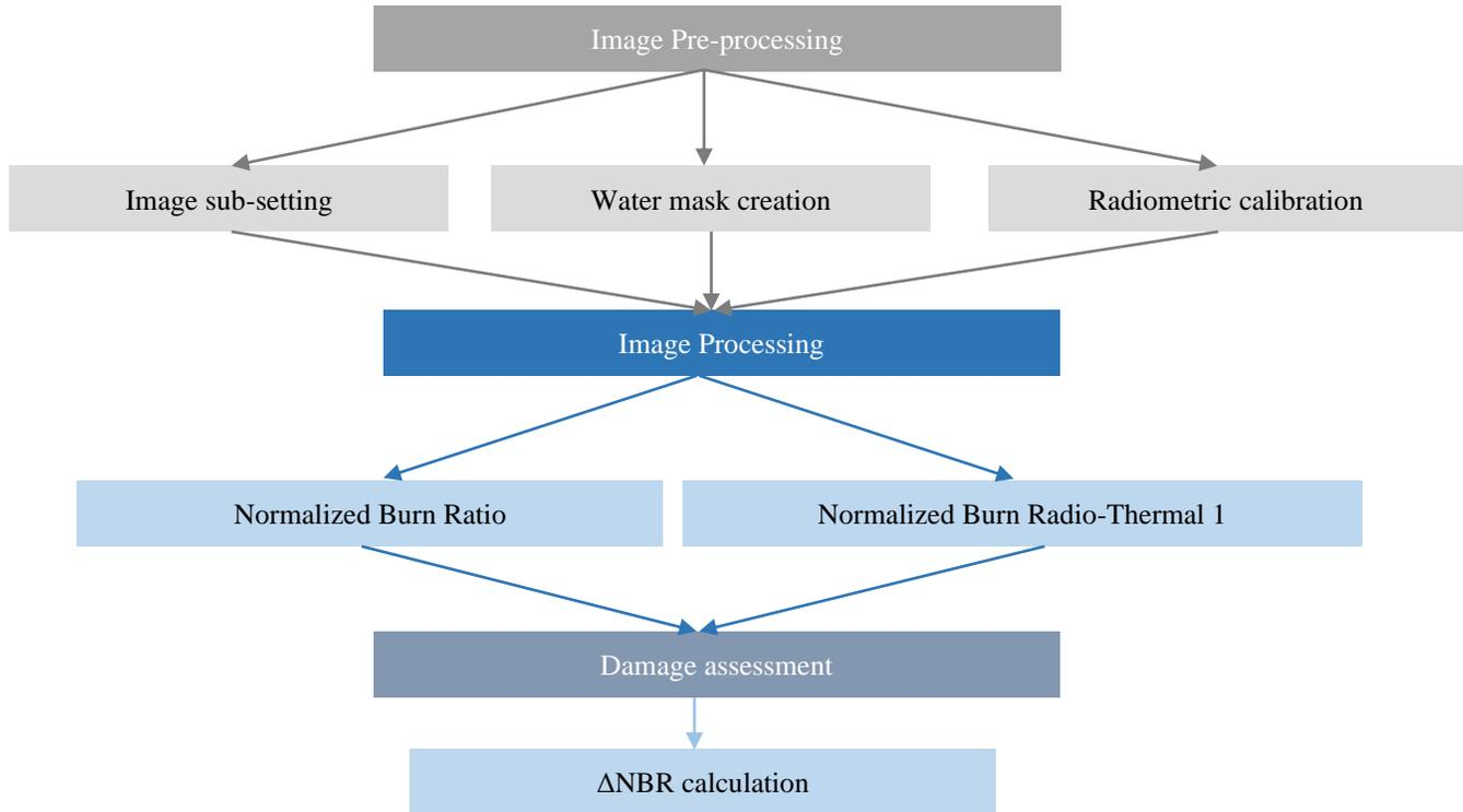
Fig. 3 Block diagram for the treatment of the images
