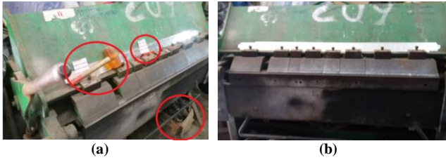
Fig. 12 Result of the application in the 1S on the bender, (a) before and (b) after.
