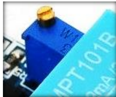
Fig. 4 Potentiometer with adjusted screw
