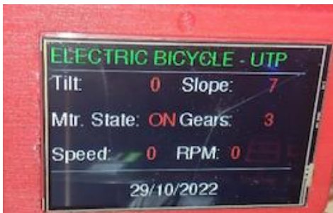
Fig. 35 Referential photo of the screen with a slope of 7°.
