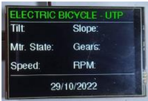
Fig. 15 Presentation on TFT LCD screen
