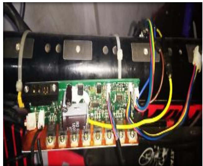
Fig. 10 Implementation of the controller with the battery
