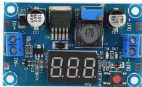
Fig. 7 Regulator switching LM2596
