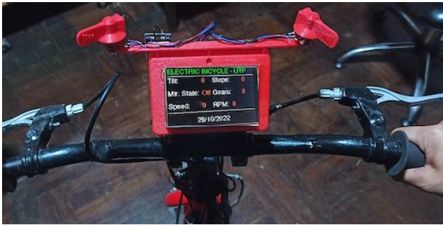
Fig. 22 Implementation of the control circuit casing
