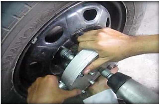
Fig. 4 Removing all wheel nuts using VAWNR and impact wrench
