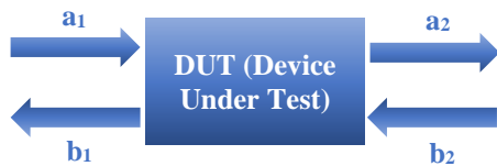
Fig. 11 Two-port network visualised with S-Parameters
