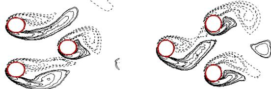
Fig. 5 Vorticity contours plot for Re = 100, T = 3D, and w = 0.25
