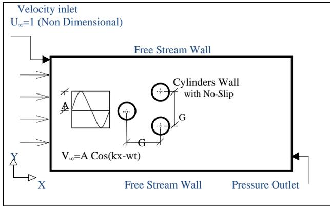
Fig. 1 (b) Physical representation of problem configuration with single cylinder upstream
