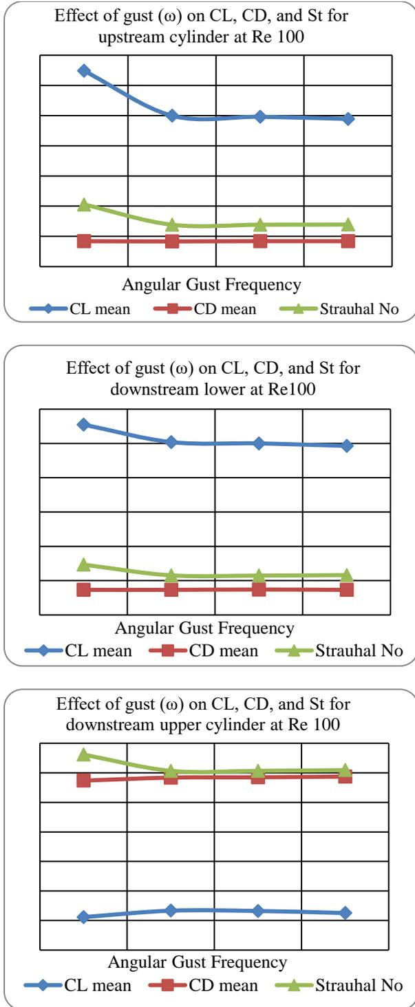
Fig. 8 Effect of gust ( $\omega$ ) on  $C_L$ ,  $C_D$ , and  $S_t$  at Re 100
