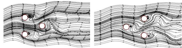
Fig. 4 Streamline plot for Re = 100, T = 3D, and w = 0.25π
