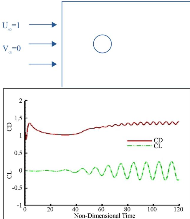
Fig. 2 Model flow problem and its  $C_L$  and  $C_D$  evolution at Re 100 [13]
