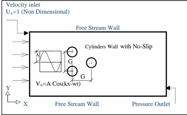
Fig. 1 (a) Physical representation of problem configuration with single cylinder downstream
