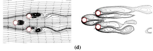
Fig. 7 Streamline plot for  $Re = 100$ ,  $T = 3D$ , and (a)  $w = 0.25\pi$ , (b)  $w = 0.50\pi$ , (c)  $w = 0.75\pi$ , (d)  $w = 1.0\pi$
