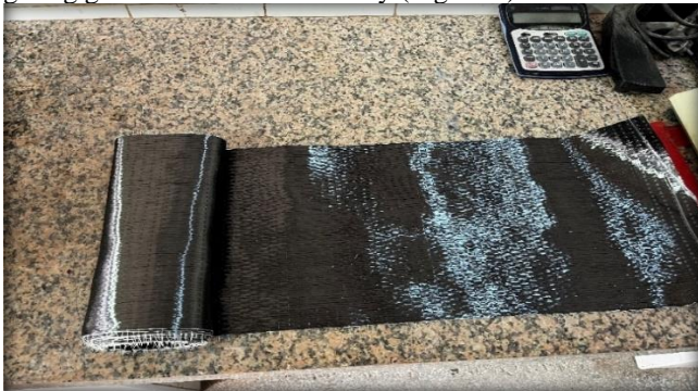
Fig. 2 CFRP Sikawrap 230C used in the experimental study
