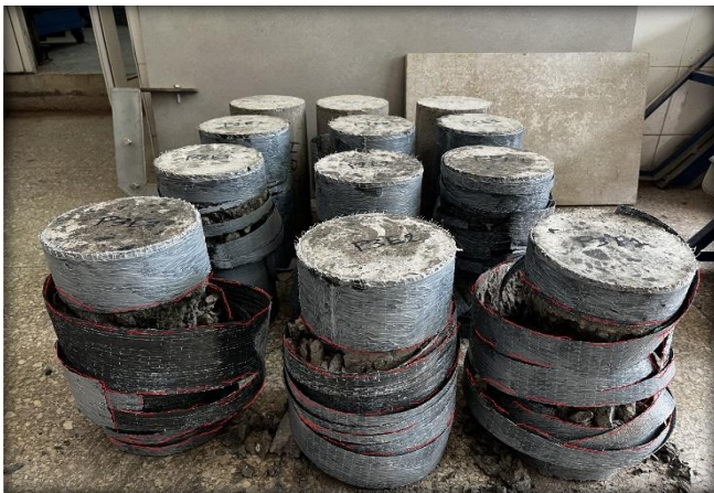
Fig. 5 Failure mode of cylindrical specimens confined with CFRP
