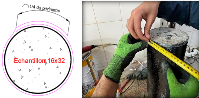
Fig. 4 Overlap length for confined circular specimen with 1 “PRF” layer
