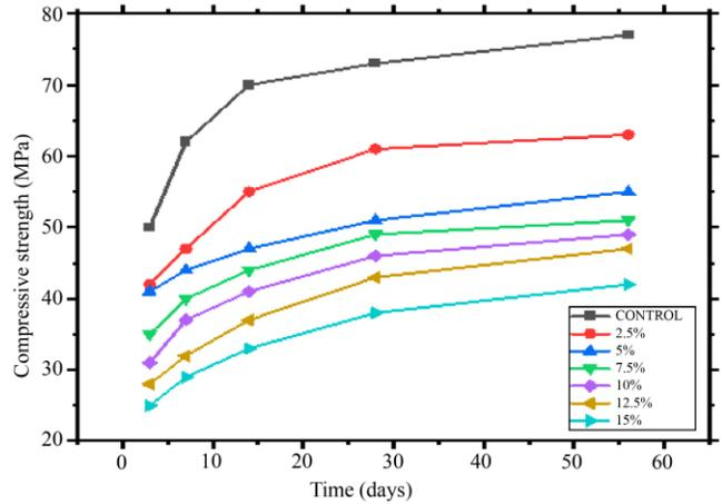
Fig. 4(b) The impact of CR particle size (0.18-1.25mm) on the compressive strength of concrete
