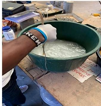
Stage 2. Preparation of NaOH solution
