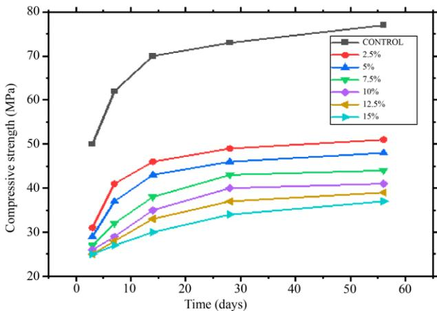
Fig. 4(a) The impact of CR particle size (0.18-5mm) on the compressive strength of concrete
