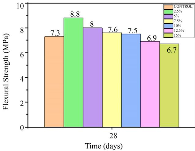
Fig. 6(a) The impact of CR particle size (0.18-5mm) on the flexural strength of concrete
