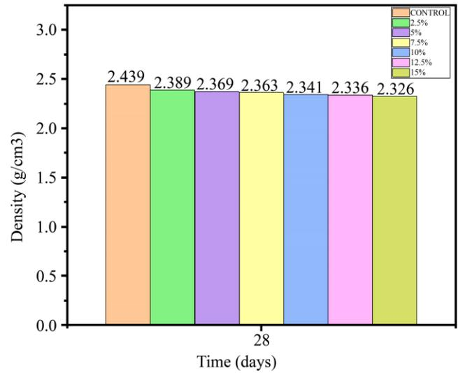
Fig. 7(b) The impact of CR particle size (0.18-1.25mm) on the density of concrete
