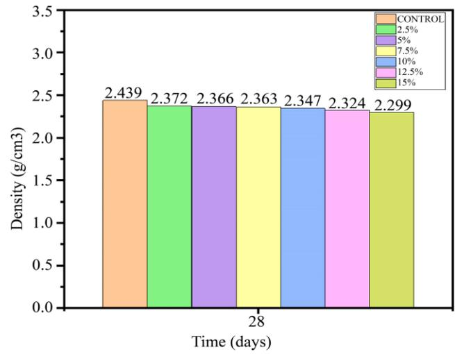
Fig. 7(a) The impact of CR particle size (0.18-5mm) on the density of concrete
