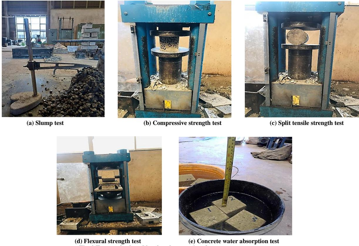
(a) Slump test (b) Compressive strength test (c) Split tensile strength test (d) Flexural strength test (e) Concrete water absorption test
