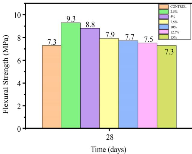
Fig. 6(b) The impact of CR particle size (0.18-1.25mm) on the flexural strength of concrete
