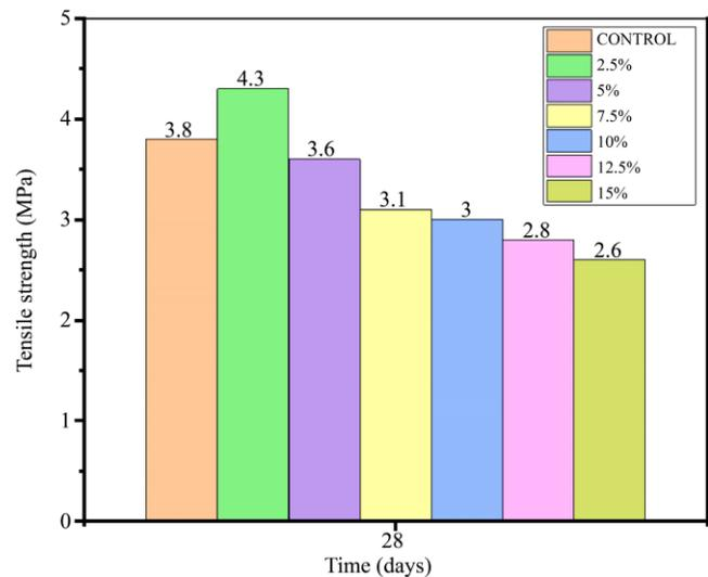
Fig. 5(b) The impact of CR particle size (0.18-1.25mm) on the tensile strength of concrete
