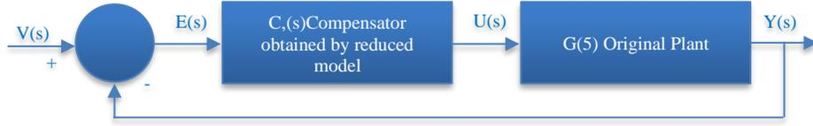
Fig. 2 Overall closed loop controlled unity feedback system with reduced order compensator
