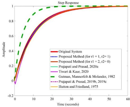
Fig. 4 Example 1- Response of SISO system for a step input
