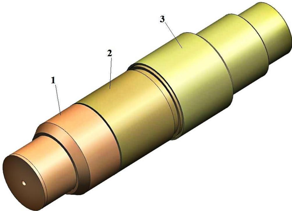
Fig. 2 The microplasma torch: 1 – anode section, 2 – cathode section, 3 – bottom section
