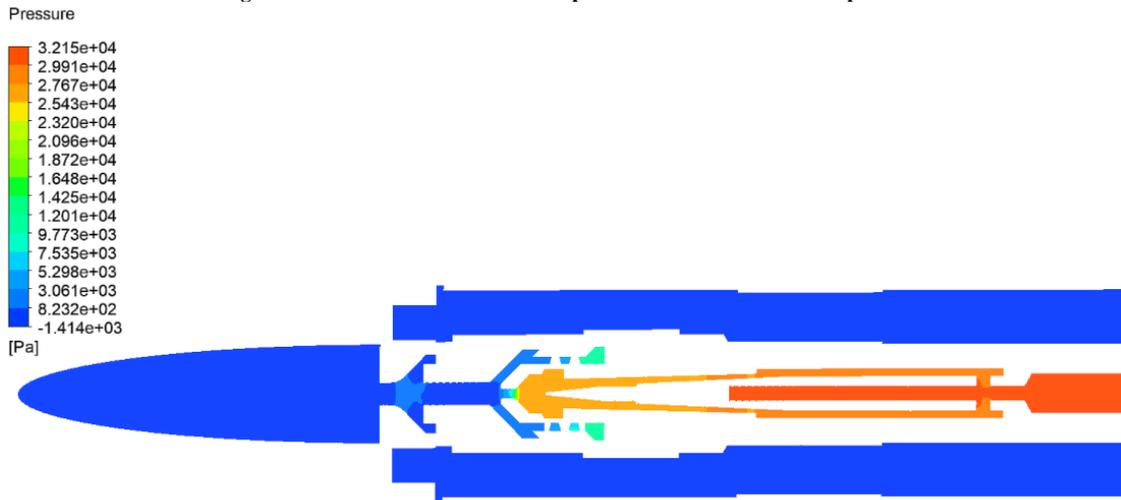
Fig. 11 Distribution of pressures in the plasma torch model in section plane A
