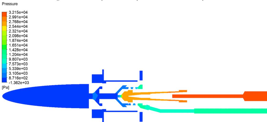
Fig. 12 Distribution of pressures in the plasma torch model in section plane B
