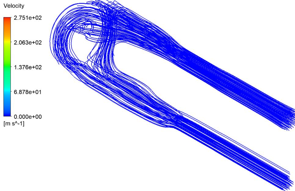
Fig. 14 Current paths in the computational domain of the coolant
