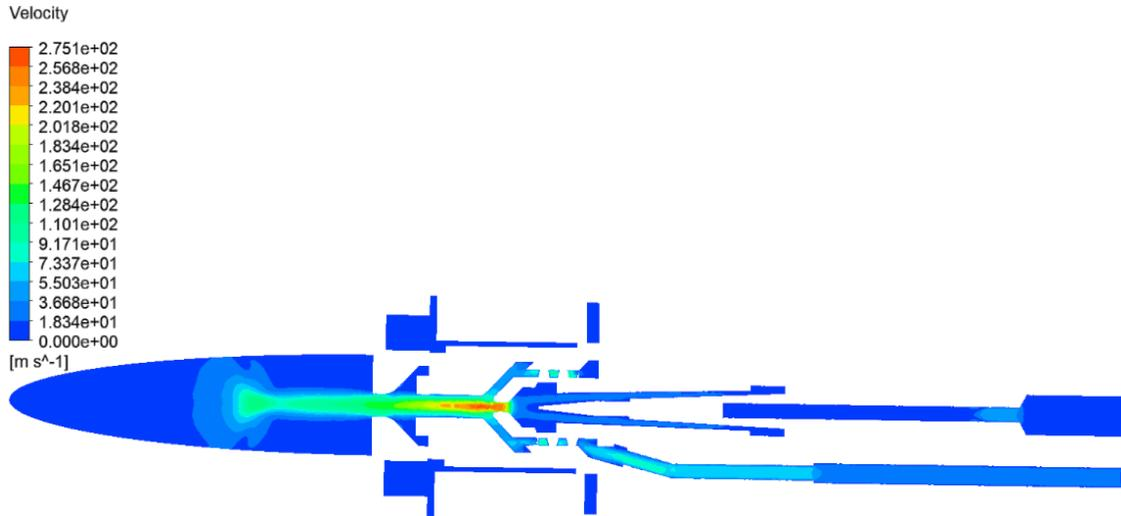
Fig. 10 Distribution of velocities in the plasma torch model in section plane B
