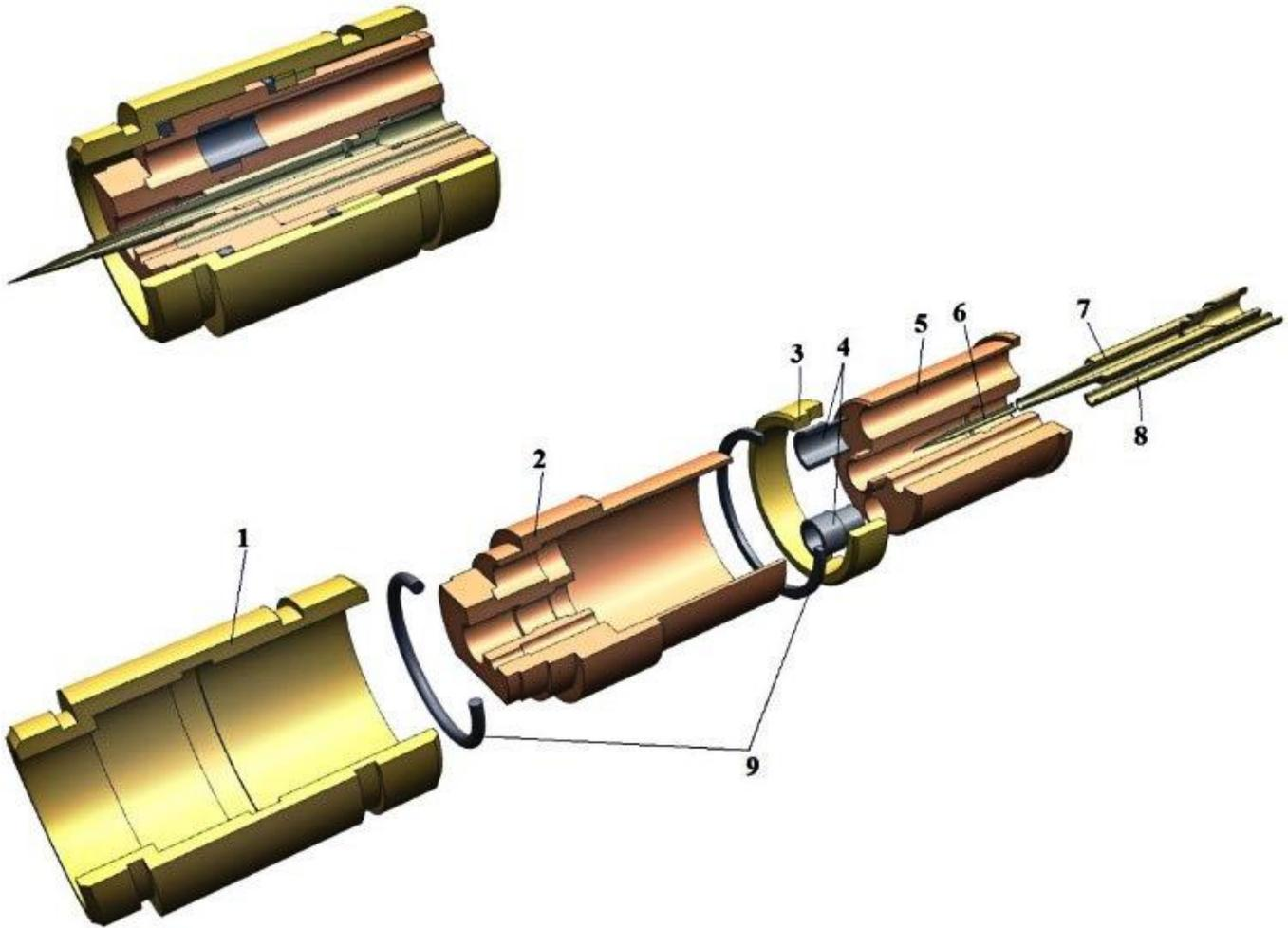
Fig. 5 The cathode section: 1 – micro plasma torch body, 2 – cathode insulator, 3 – internal nut, 4 – water sleeve, 5 – cathode body, 6 – tip, 7 – cathode holder, 8 – powder supply tube, 9 – O-rings
