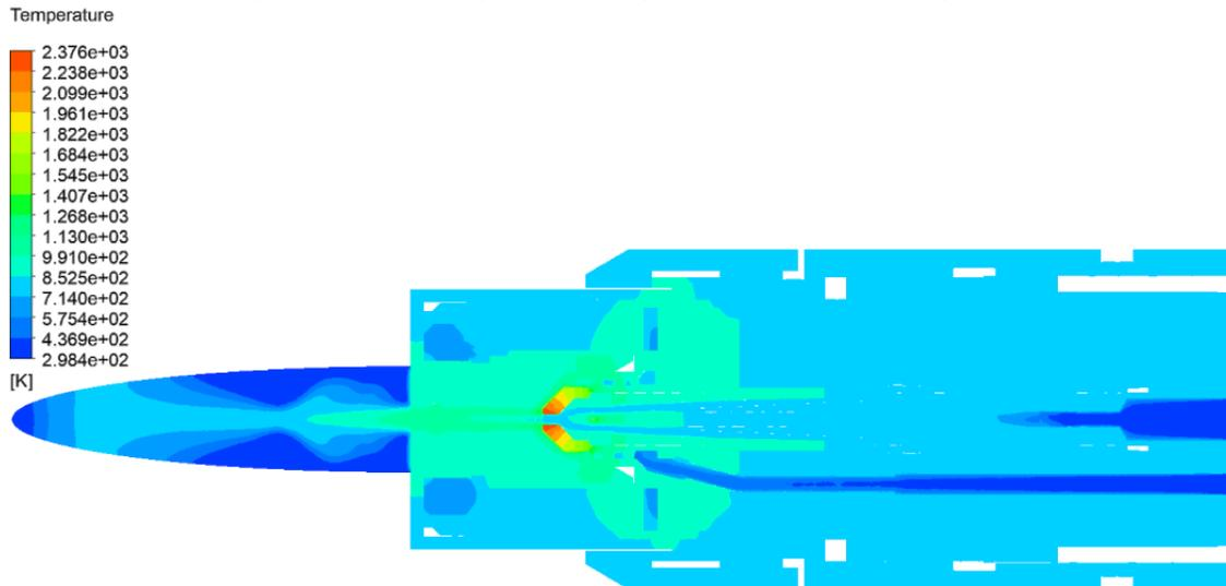
Fig. 8 Distribution of temperatures in the plasma torch model in section plane B
