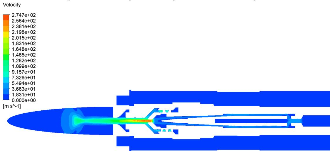
Fig. 9 Distribution of velocities in the plasma torch model in section plane A
