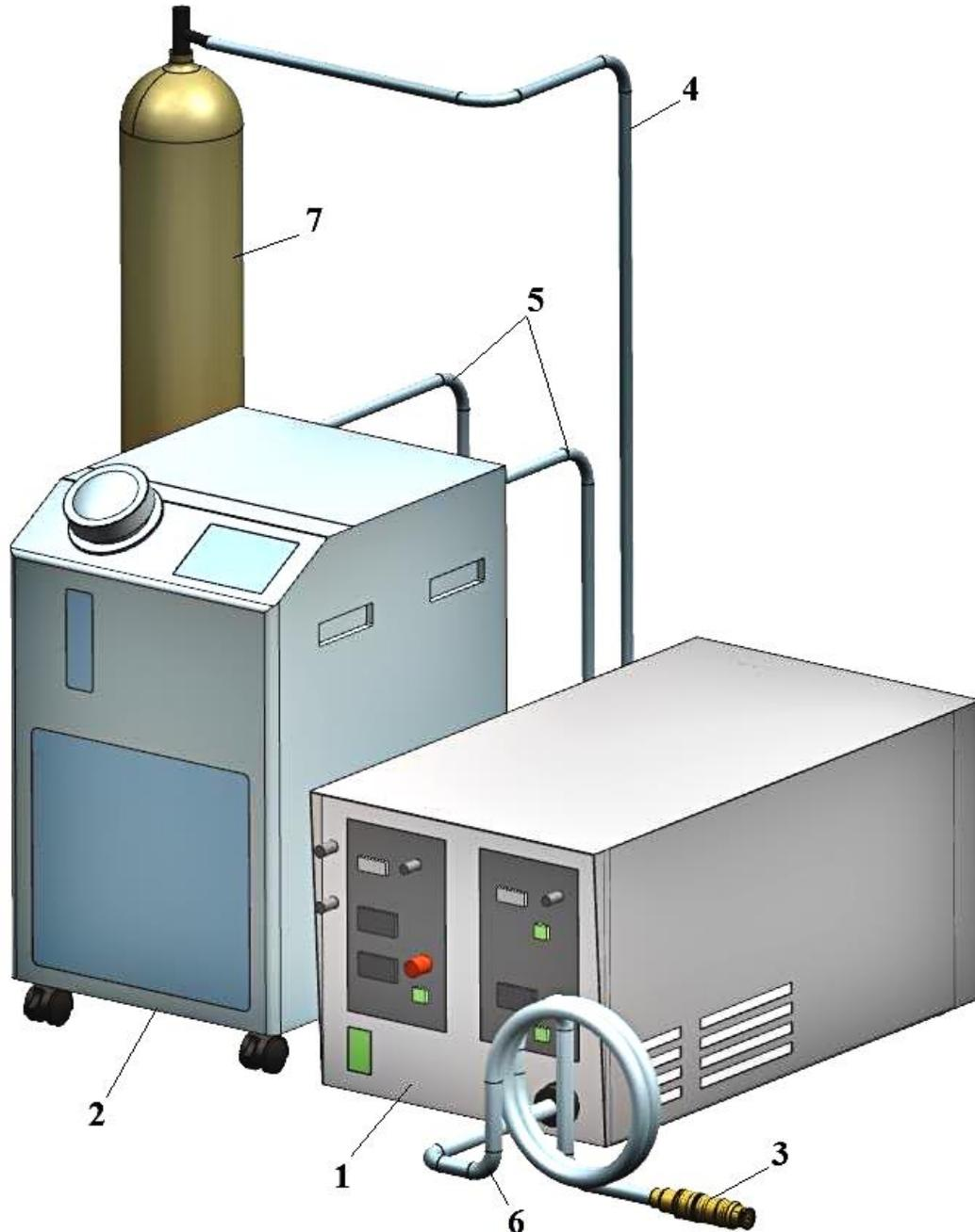
Fig. 1 The IFPCU design: 1 – maintenance section, 2 – cooling section, 3 – micro plasma torch, 4 – gas hose, 5 – water hose, 6 –plasma torch supply hose, 7 – gas cylinder
