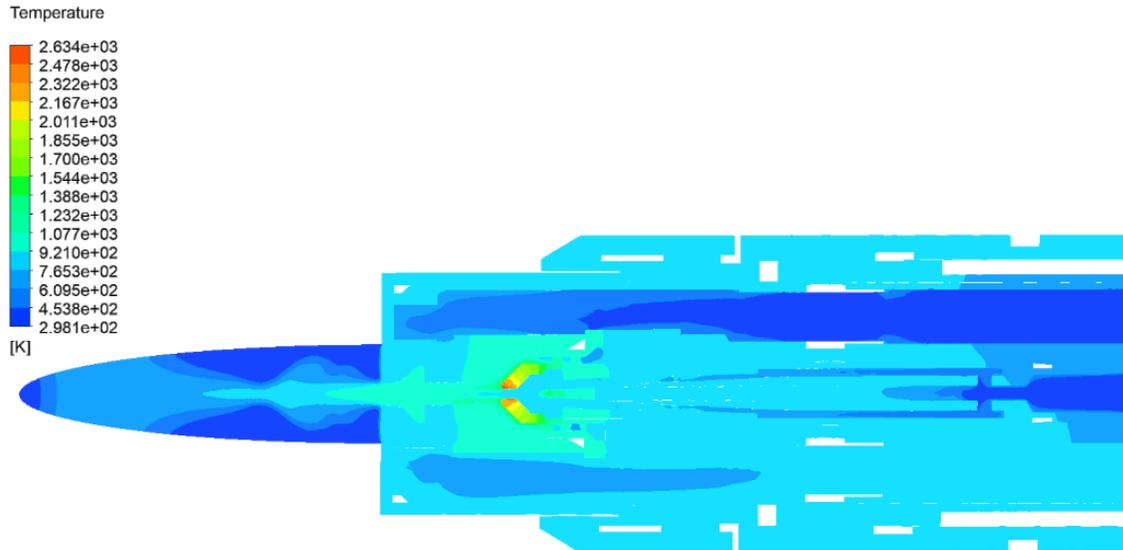
Fig. 7 Distribution of temperatures in the plasma torch model in section plane A
