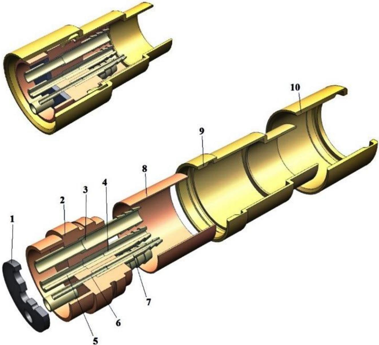
Fig. 4 The bottom section: 1 – gasket, 2 – base plug, 3 – water cooling fitting, 4 – gas supply fitting, 5 – gas supply fitting tube, 6 – powder supply fitting tube, 7 – powder supply fitting, 8 – tube, 9 – housing, 10 – cup
