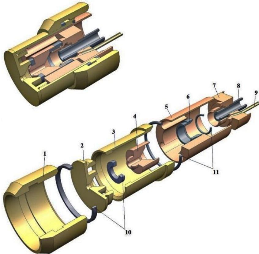
Fig. 3 The anode section: 1 – union nut, 2 – anode holder, 3 – anode body, 4 – output section of the interelectrode insert (IEI), 5 – insert insulator, 6 – IEI bushing, 7 – IEI input section, 8 – bushing, 9 – tube, 10 – insulating rings, 11 – sealing rings
