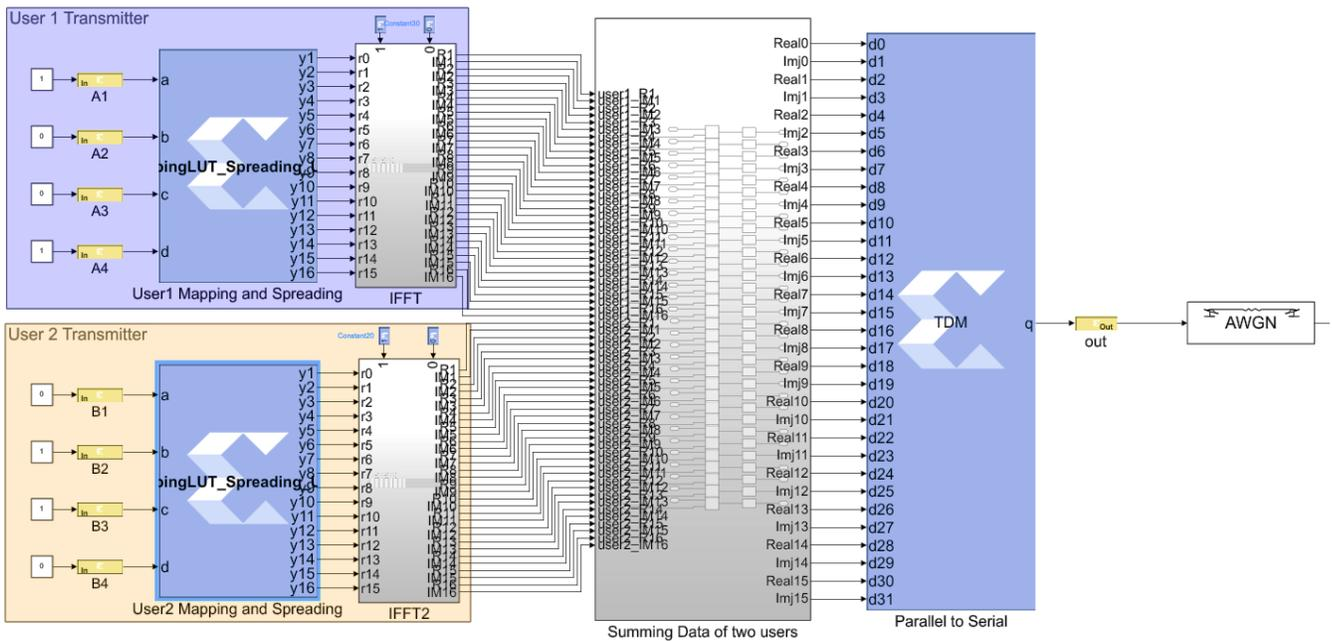
Fig. 5 System generator simulink of the enhanced MC-MC-CDMA transmitter for  $M=16$
