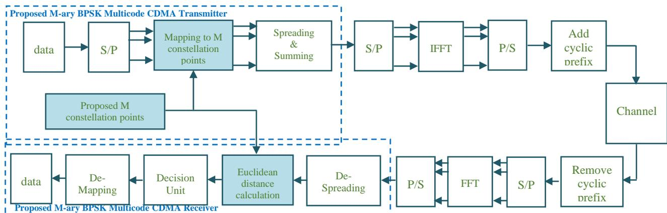
Fig. 2 The enhanced MC-MC-CDM system model
