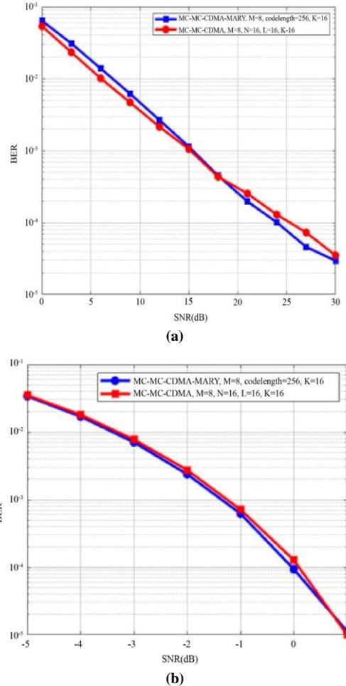
Fig. 12 Comparison of MC-MC-CDMA and the enhanced MC-MC-CDMA for 8-ary and 16 users in (a) Fading channel (b) AWGN channel
