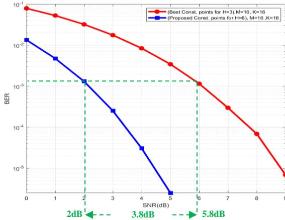
Fig. 9 Comparison of the proposed 16-ary BPSK Multicode CDMA for proposed points of H=8 and best constellation points of H=3
