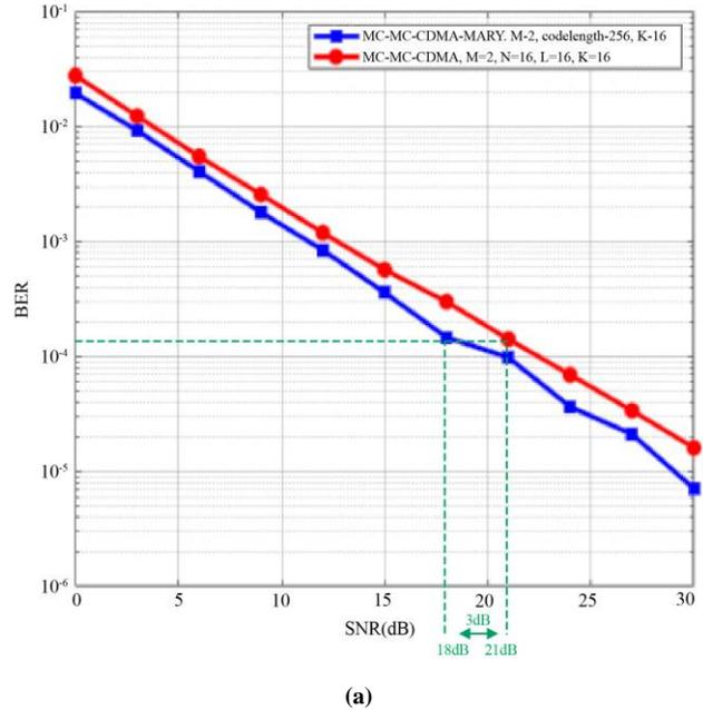
Fig. 13 Comparison of MC-MC-CDMA and the enhanced MC-MC-CDMA for M=4 and 16 users in (a) Fading channel (b) AWGN channel
