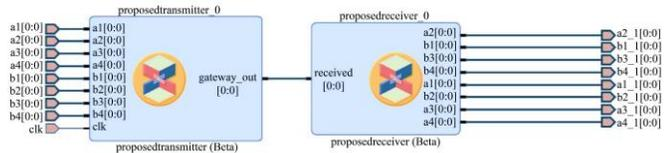
Fig. 8 VIVADO block design of the proposed MC-MC-CDMA
