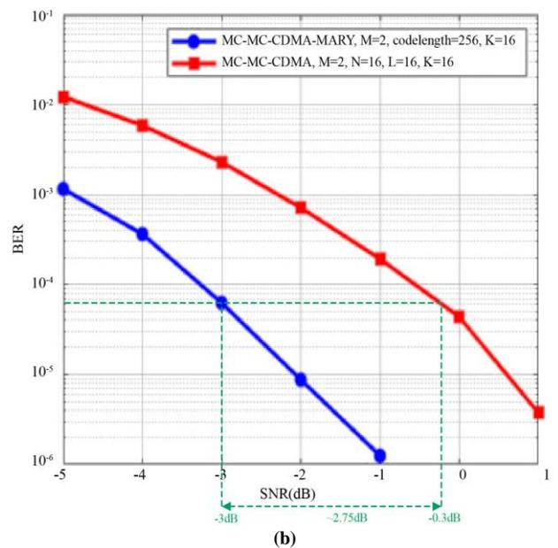
Fig. 14 Comparison of MC-MC-CDMA and the enhanced MC-MC-CDMA for M=2 and 16 users in (a) Fading channel (b) AWGN channel
