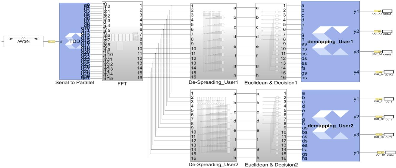
Fig. 6 System generator simulink of the enhanced MC-MC-CDMA receiver for M=16
