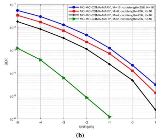
Fig. 10 BER with SNR for the enhanced MC-MC-CDMA with different M and 16 users in (a) Fading channel (b) AWGN channel
