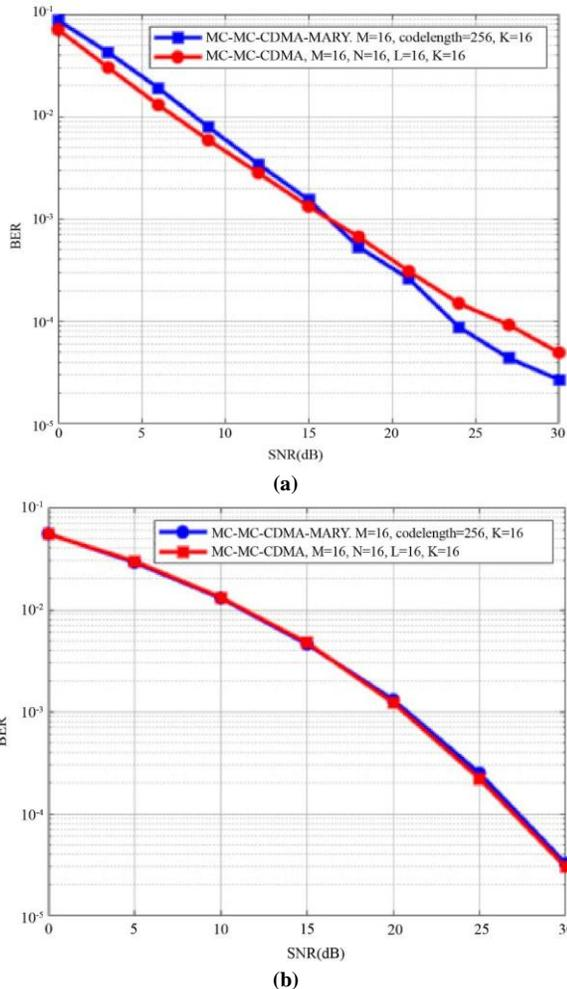
Fig. 11 Comparison of the enhanced and classical MC-MC-CDMA for 16-ary and 16 users in (a) Fading channel (b) AWGN channel
