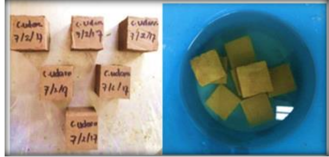
Fig. 1 Treatment process (curing) of the test object
