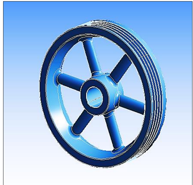
Fig. 9 Optimized flywheel geometry
